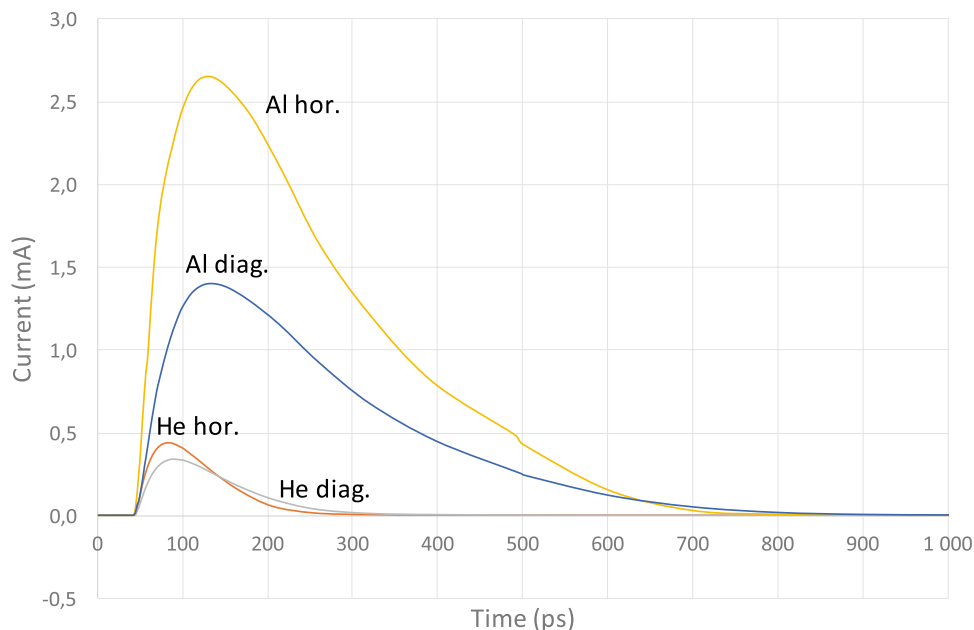
Fig. 7 Currents generated by Alpha and Aluminum particles in two different configurations: horizontal (hor.) and diagonal (diag.)
