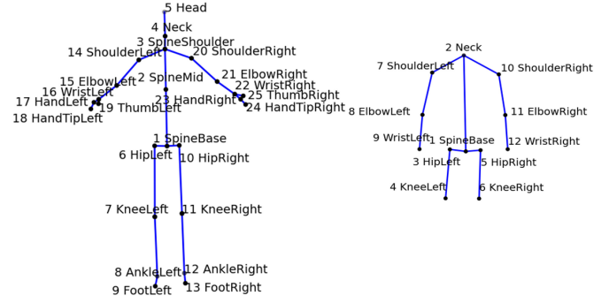
Figure 1. Joints differences between a complete pose of 25 joints (left) and a partial pose of 12 joints (right).
