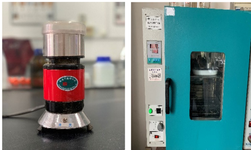
(a) The high speed universal disintegrator. (b) Electric thermostat blast drying oven.
