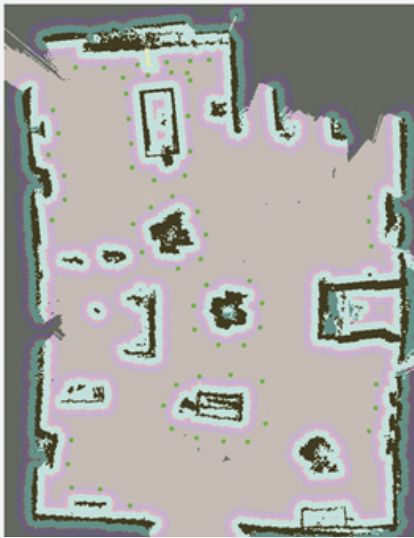
Figure 6: An example of the global path, the green points indicate discrete destinations that cover all the target area.
