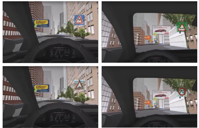
Fig. 2. The screenshots of our implemented driving simulation testbed [20] with synthetic traffic signs generated by the proposed generative diffusion model, named TSDreamBooth.
