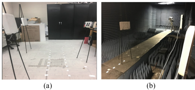
Fig. 9. Setup of two experimental scenarios for SparseTag performance evaluation. (a) Computer lab setup. (b) Anechoic chamber setup.
