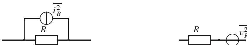
Figure 23: Two equivalent ways of depicting the noise sources of a resistor. Left a current noise source (parallel to the resistor). Right a voltage noise source (in series with the resistor).
