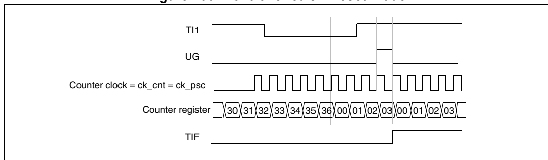
Figure 200. Control circuit in reset mode
