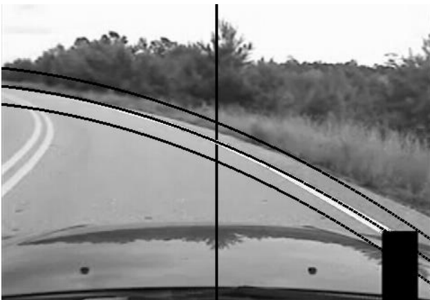
Figure 7: Interpolated polynomial with bounds for the right lane marking
