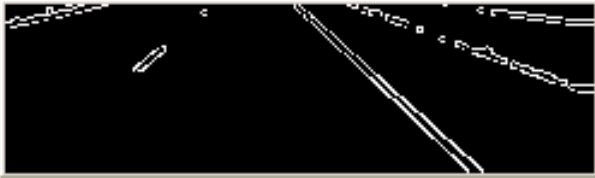
Figure 2: Image on highway following edge detection
