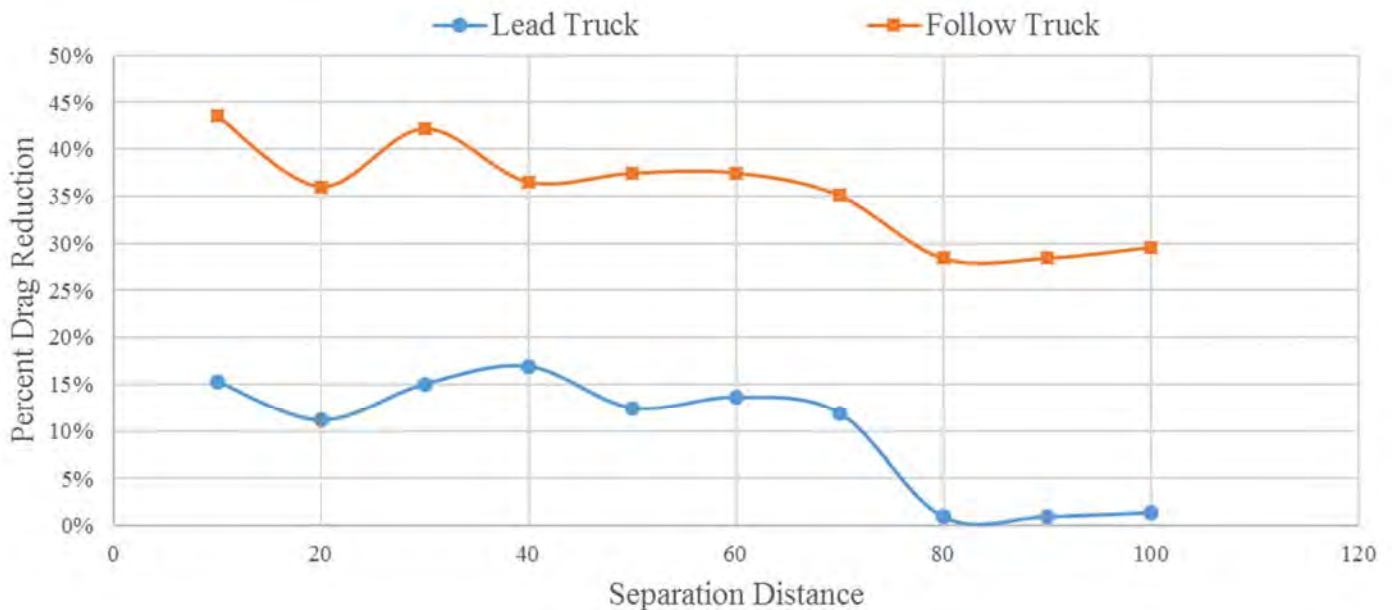
Figure 37: Drag reduction vs. separation distance for centered 5mph crosswind
