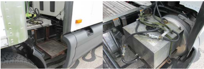
Figure 84: Left: Auxiliary tank mount Right: Auxiliary tank secured to mount and connected to fuel supply and return fuel lines
