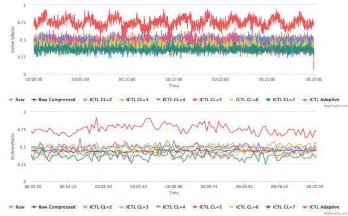
Figure 34: ADR from adaptive ICTL compared other transmission strategies with 12 nodes: 30-minute view and 2-minute zoom-in view
