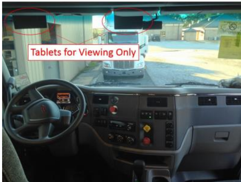
Figure 6: Installation of Tablets for Human-Machine Interface
