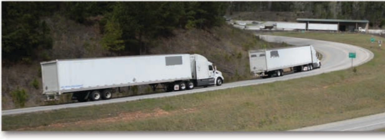
Figure 9: Peterbilt 579 Tractors in Platoon Utilizing Peloton's Prototype DATP System
