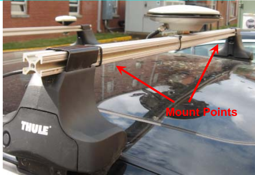
Figure 5: Auburn Engineering Vehicle Test Platform roof rack and mount points for Sarnoff Sensor Bar
