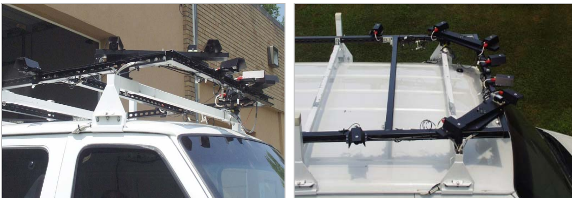
Figure 3: Multi-camera system mounted on a van. The system include 2 stereo pairs, 4 monocular cameras, IMU and GPS
