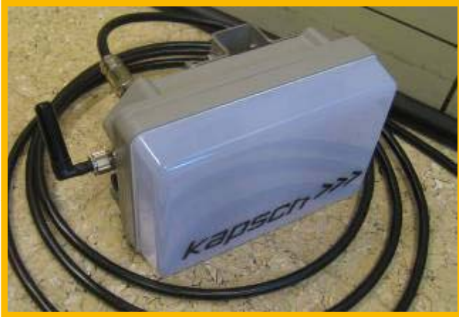
5.9GHz Roadside Communication Equipment
