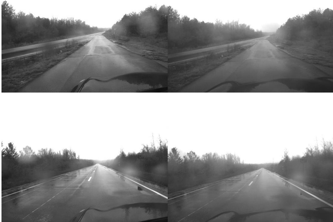
Figure 12: Image samples from front stereo pair. Rain caused image blur and specularities. Fogging of right image was caused by condensation between CCD and lens.
