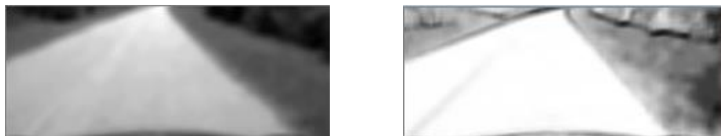
Figure 79: Unnormalized Correlation Matching (left) and Normalized Correlation Matching (right)
