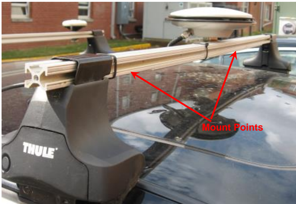
Figure 6: Auburn Engineering Vehicle Test Platform roof rack and mount points for SRI Sarnoff sensor bar
