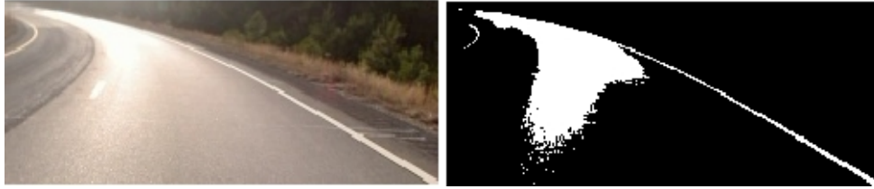
Figure 16: Reflection of sun in road (left) and corresponding edge map with constant threshold (right)
