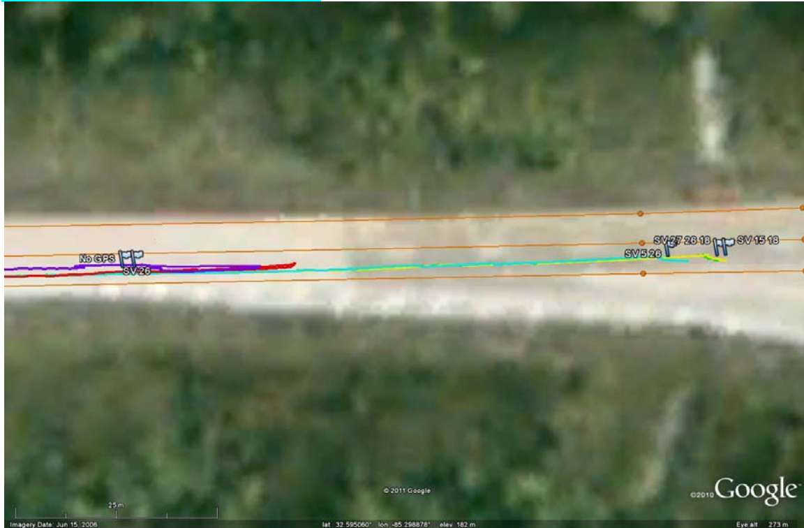
Figure 56: Estimated North-East Position with Vision Measurements, Map, and Limited Satellite Visibility
