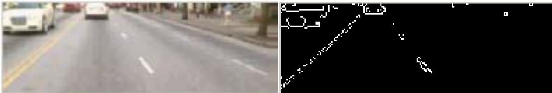
Figure 18: City street (left) and corresponding edge map (right)
