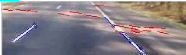
Figure 6: Lines from the Hough Transform- pass (blue) and fail (red)
