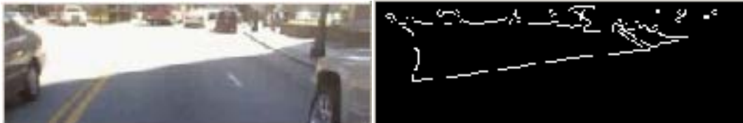
Figure 20: Sunlight peering between buildings (left) and corresponding edge map (right)
