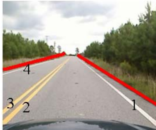
Figure 2.8: Corresponding echo width to lane markings [1]
