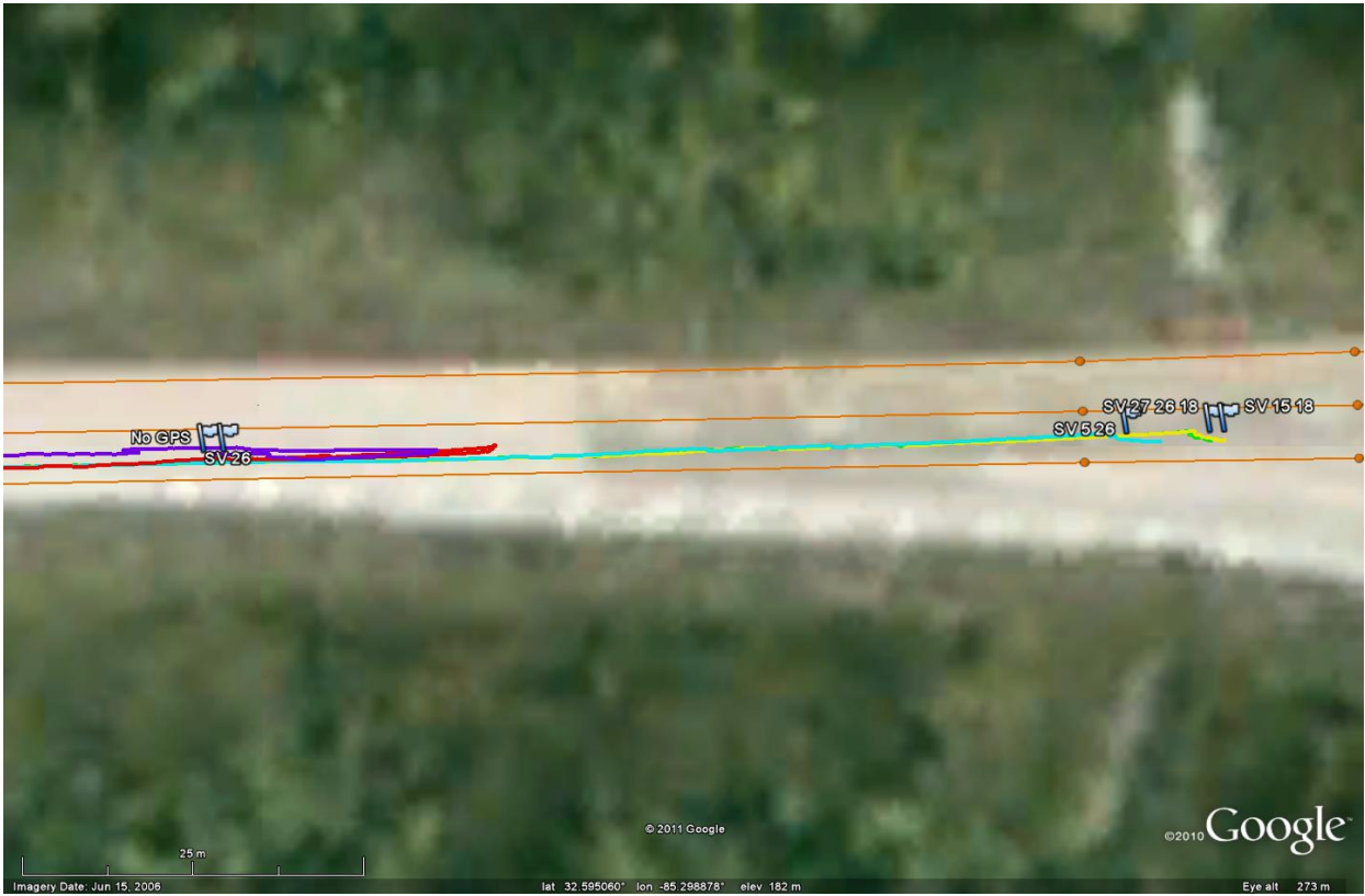
Figure 5.17: Estimated North-East Position with Vision Measurements, Map, and Limited Satellite Visibility
