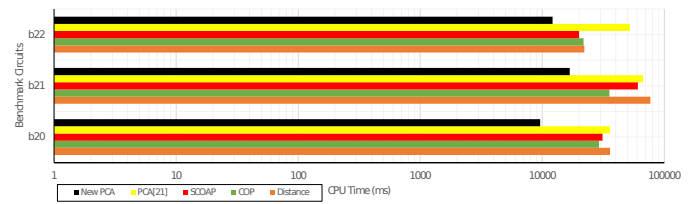
Fig. 8. Total ATPG CPU time for finding a test or proving redundancy for 100 hard-to-detect faults in three ITC’99 [36] benchmark circuits.
