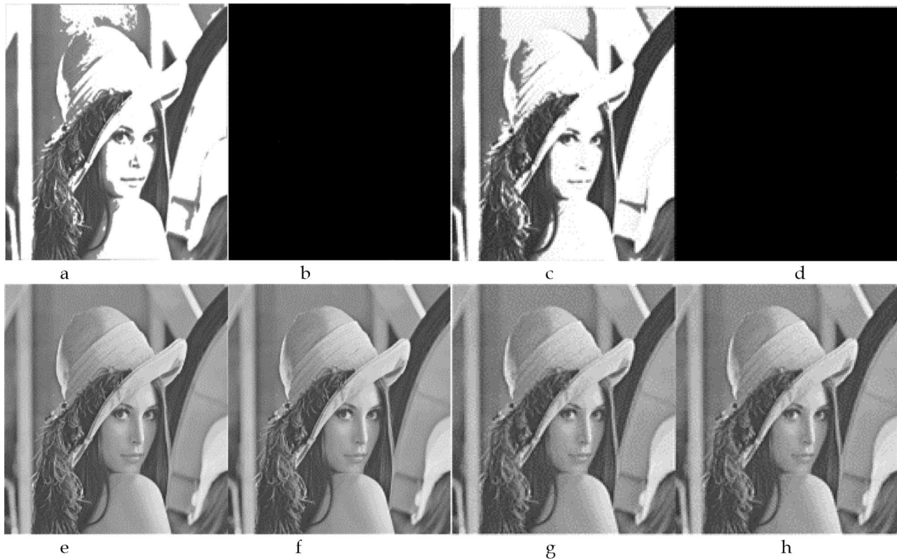
Fig. 10 Outputs with Lena as the input image. a Architecture 1 with single stuck-at-0 fault. b Architecture 1 with single stuck-at-1 fault. c Architecture 2 with a single stuck-at-0 fault d Architecture 2 with
