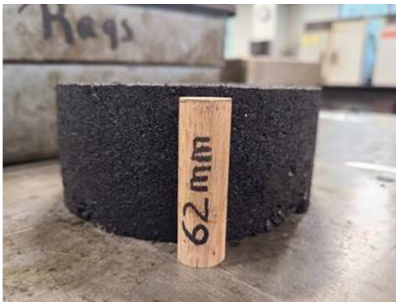
FIGURE 15 Typical expansion with RTR specimens.
