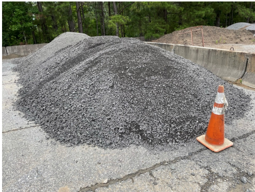
FIGURE 3 Stockpiled reclaimed CCPR millings.
