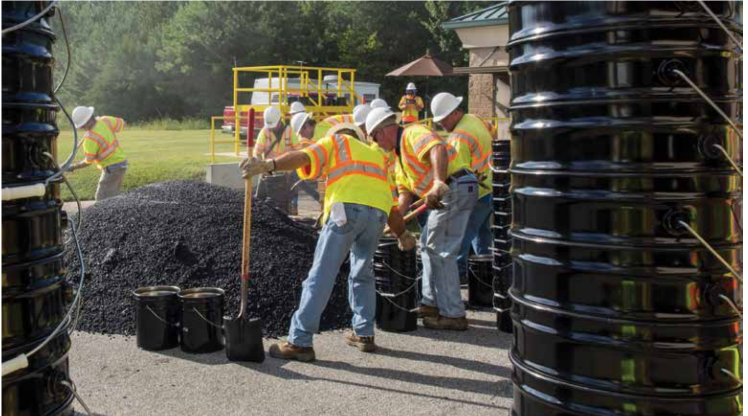
Two hundred five-gallon buckets of asphalt mix were sampled during 2018 Test Track construction for the round-robin study.
