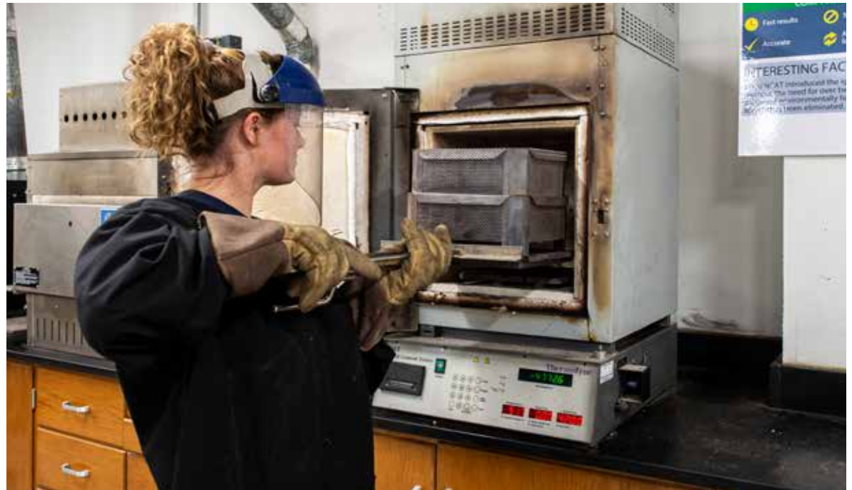
Developed at NCAT, the ignition oven set the industry standard for determining asphalt content by ignition method.
