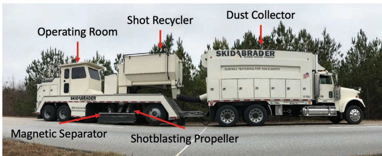
Shotblasting system on Section W5 at the NCAT Test Track.
