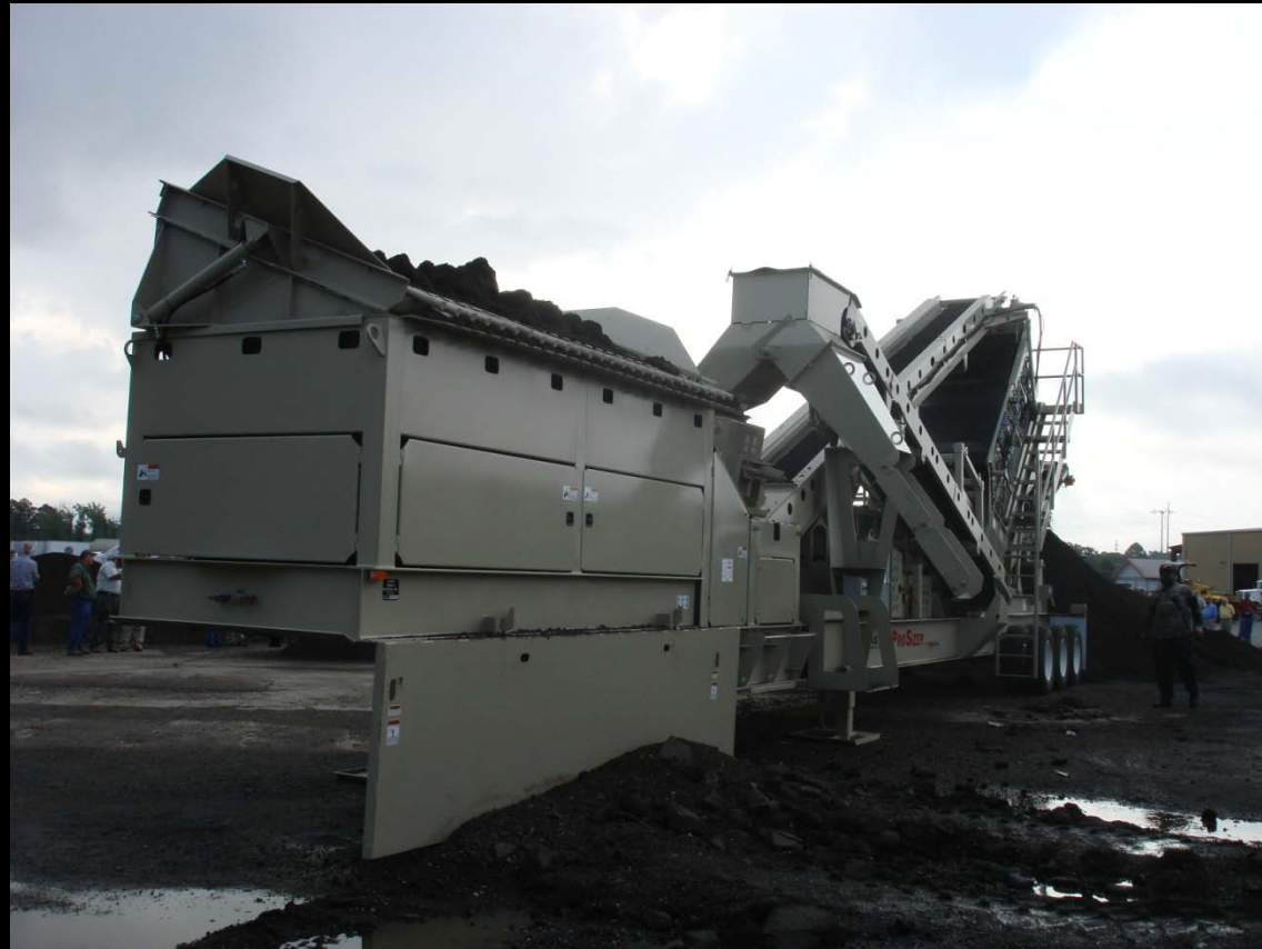
RAP Sizing Plant
