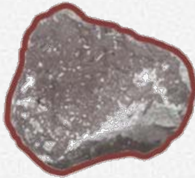
HARDER LIQUID TRANSFERRED FROM RAP PREVENTS STRIPPING
