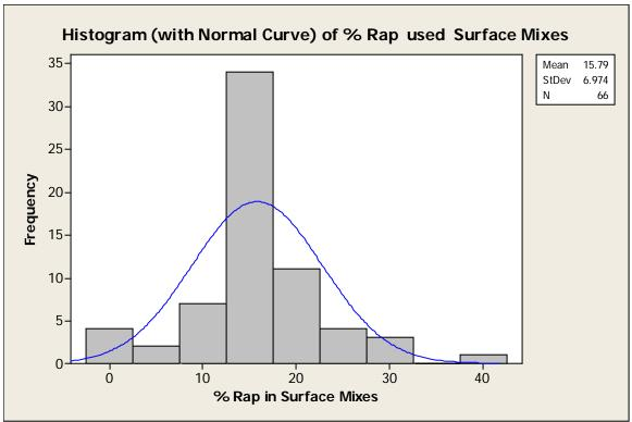
Figure 5. Histogram of Typical % RAP Used in Surface Mixes
