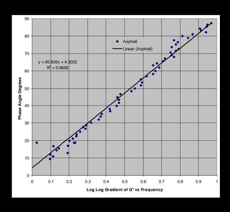
Rowe determined linear relationship between phase angle and log log slope of G\* vs freq
