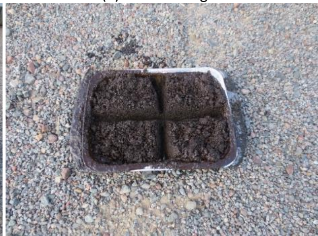
(f) Quartered sample ready for testing
