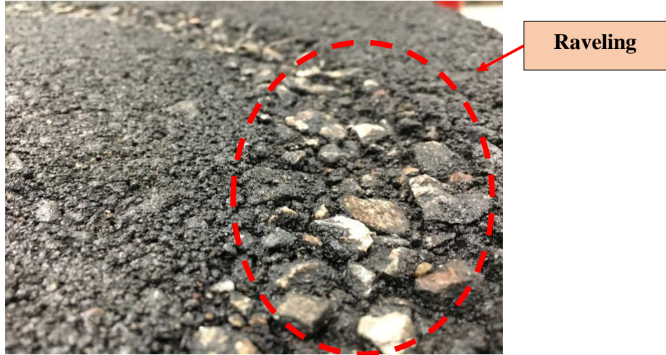
Figure 3. Polished Slab of Mix BMN
