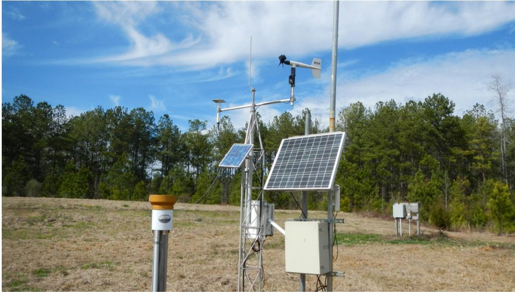
**Figure 28 Test Track On-Site Weather Station**
