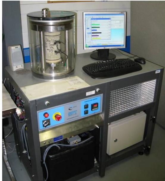
**Figure 18 IPC Global Asphalt Mixture Performance Tester**
