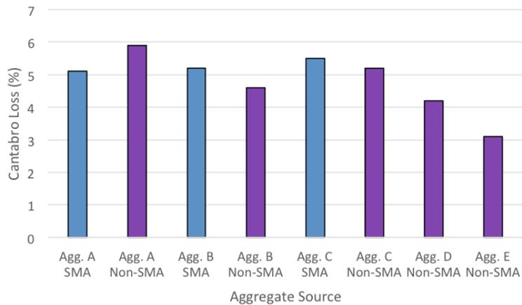
**FIGURE 5 Cantabro Stone Loss Based on Aggregate Source**
