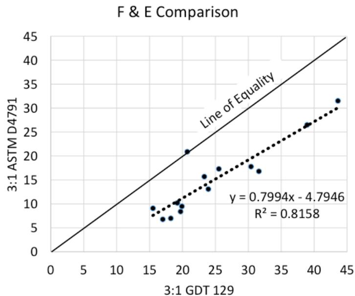
**FIGURE 1 Comparison of GDT 129 versus ASTM D4791 for 3:1 Ratio**
