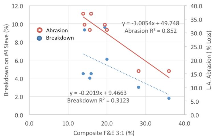
**FIGURE 3 Comparison of the Effect of F&E on Aggregate Breakdown and L.A. Abrasion**
