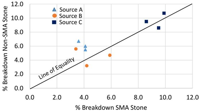
**FIGURE 2 Comparison of Aggregate Breakdown on the No. 4 Sieve**
