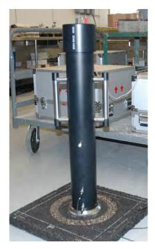
Figure 3 Impedance Tube
