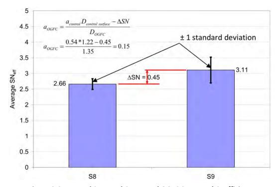
Figure 2 Computed SN<sub>eff</sub> and Computed OGFC Structural Coefficient
