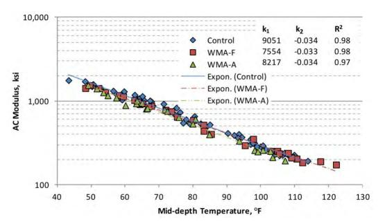
Figure 13 Backcalculated AC Modulus Versus Temperature
