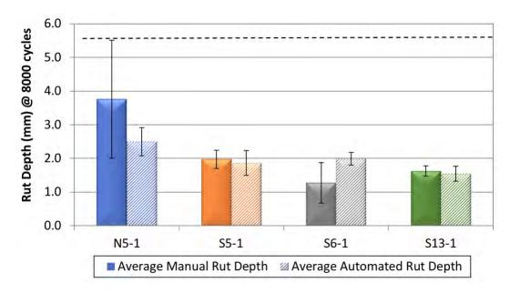
Figure 2 Asphalt Pavement Analyzer Test Results for Green Group Surface Layers
