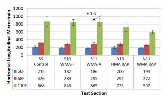
**Figure 11 Average Longitudinal Strains at Reference Temperatures**
