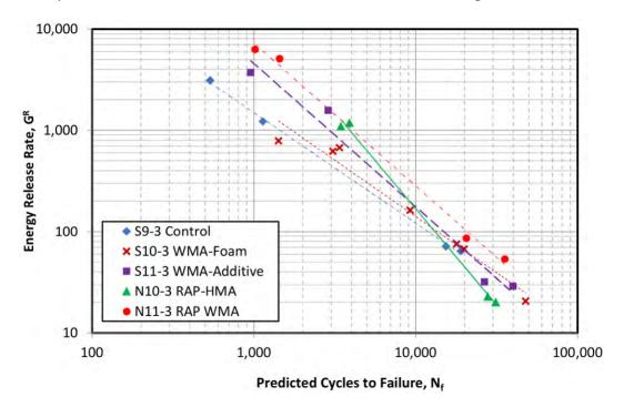
Figure 27 Predicted SVECD Cycles to Failure for GE Base Layer Mixes
