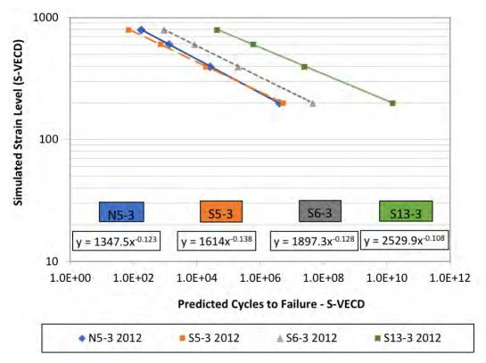
Figure 8 Fatigue Lives of Bottom Layer Mixes from SVECD Testing and Analysis
