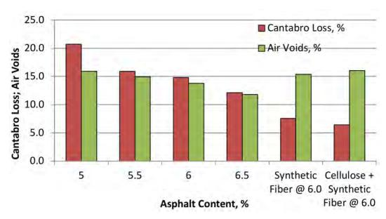
Figure 3 Effect of Fiber with 12.5 mm NMAS PFC
