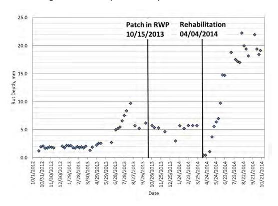
Figure 10 Section N5 (Standard RAP) Rutting Performance
