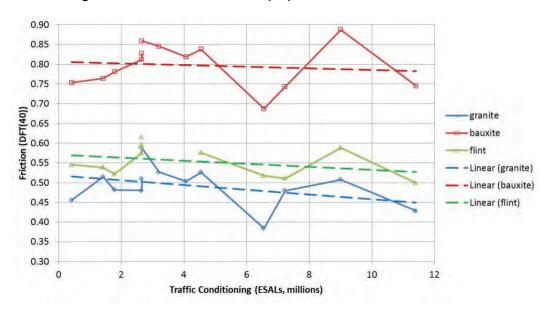
Figure 4 Left Wheel Path DFT(40) Results After 10M ESALs
