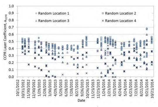
Figure 13 Structural Coefficient vs. Date/Traffic for Section N3
