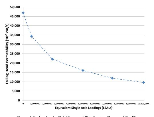
Figure 3 Reduction in Field Permeability Due to Time and Traffic
