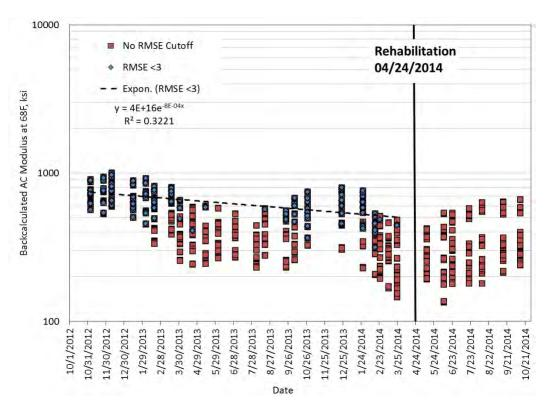
Figure 39 Section S13 (GTR) Backcalculated FWD Results
