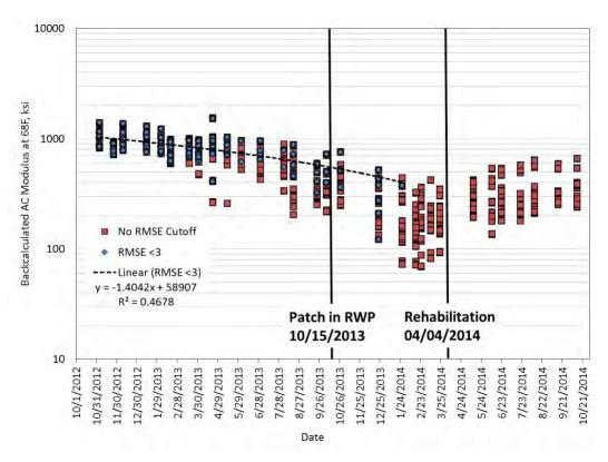
Figure 14 Section N5 (Standard RAP) Backcalculated FWD Results
