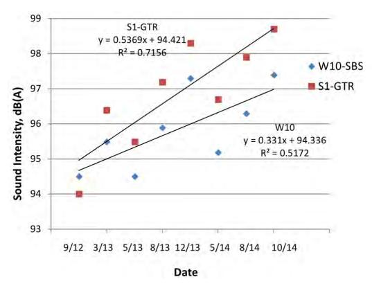
Figure 1 Section W10 & S1 OBSI Global Average Noise Measurements
