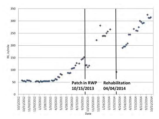
Figure 11 Section N5 (Standard RAP) Surface Performance
