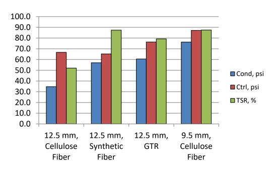
Figure 5 Comparison of Tensile Strength for ALDOT PFC
