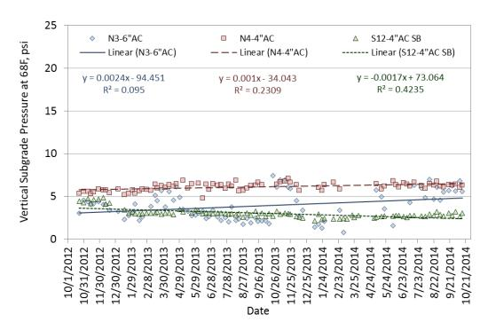
Figure 11 Subgrade Pressure at 68°F vs. Time/Traffic
