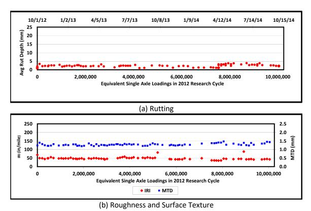
Figure 3 Rutting and Surface Texture Measurements for Section E1B
