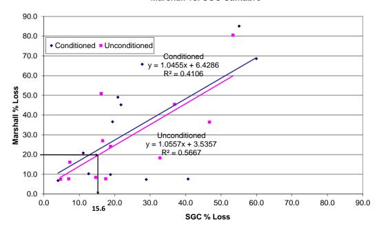
Figure 1 Comparison of Cantabro Stone Loss for Marshall vs Gyratory Samples
