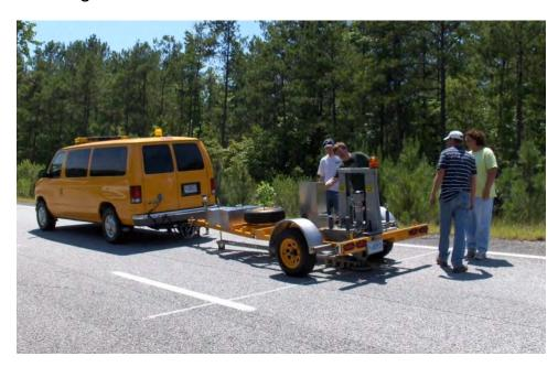
Figure 7 Dynatest Model 8000 Falling Weight Deflectometer on the Test Track
