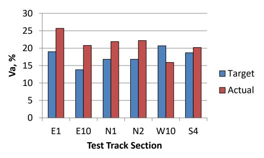
Figure 5 Mix Design vs. In-Place Air Voids
