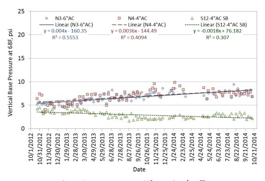
Figure 9 Base Pressure at 68°F vs. Time/Traffic
