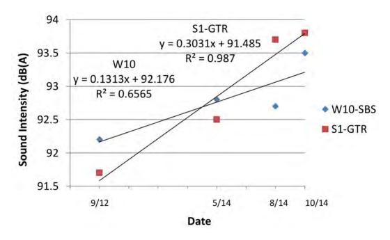
Figure 2 Section W10 & S1 CPX Global Average Noise Measurements
