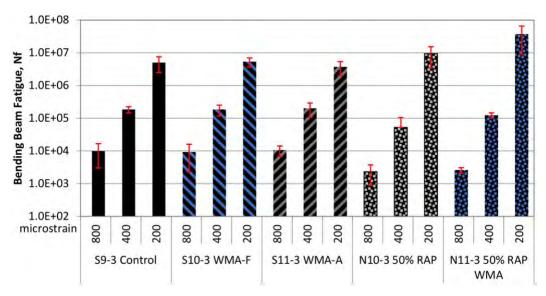
Figure 21 Bending Beam Fatigue Results for GE Base Layer Mixes
