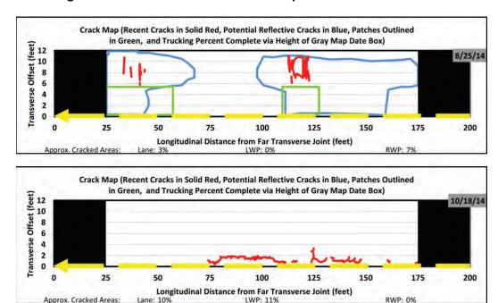
Figure 5 Cracking in Sections N8 (Top) and N9 (Bottom)
