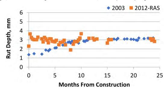
Figure 1 Rutting Comparison of 2003 OGFC vs 2012 OGFC with RAS in Section S4
