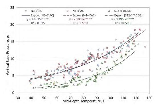
Figure 8 Base Pressure vs. Temperature
