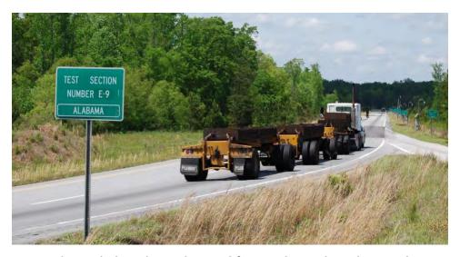
Figure 4 Heavily Loaded Triple-Trailer used for Accelerated Loading on the Test Track
