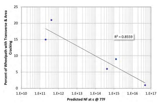
Figure 26 Relationship Between Predicted OT  $N_f$  at  $\epsilon_{77}$  and Percent of Wheelpath with Transverse and Area Cracking for GE
