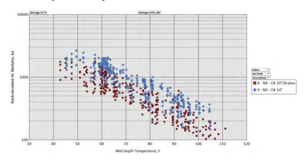
Figure 6 Backcalculated AC Modulus Versus Temperature
