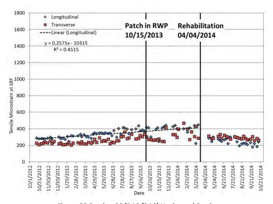
Figure 29 Section S6 (RAP/RAS) Horizontal Strain
