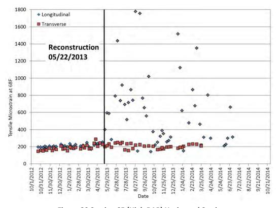
Figure 20 Section S5 (High RAP) Horizontal Strain
