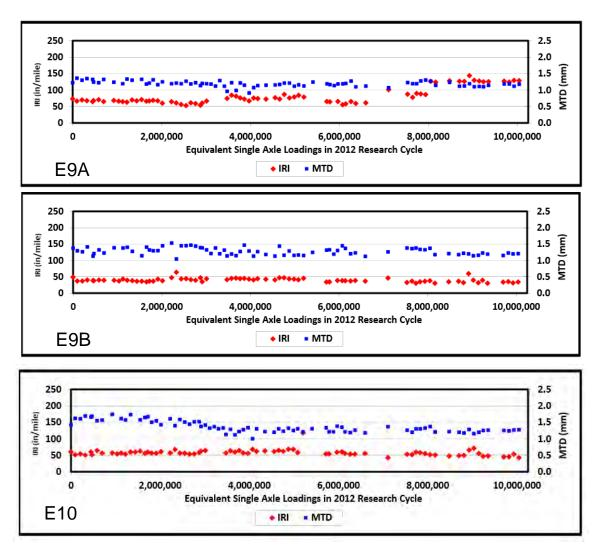
**Figure 6 Performance Comparison of ALDOT Sections**
