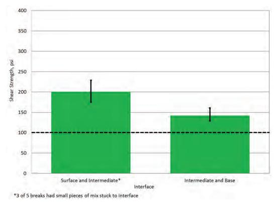
Figure 32 Bond Strength Testing Results for Section S6 (RAP/RAS)
