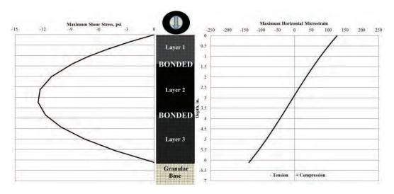
Figure 33 (a) WESLEA Simulation of Section S6 (RAP/RAS) in Fully Bonded Condition (1)
