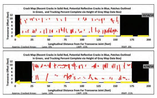
Figure 4 Crack Maps for HiMA in October 2014 (Top) and Control (Bottom) in April 2014
