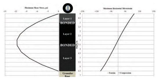
Figure 23 (a) WESLEA Simulation of Section S5 (High RAP) in Fully Bonded Condition (1)
