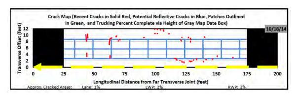
Figure 2 Crack Map of N12 (Double Surface Treatment Interlayer)
