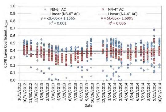
Figure 12 Structural Coefficient vs. Date/Traffic
