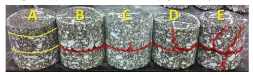
Figure 22 (b) Cores Taken from Section S5 (High RAP) in April 2013 (Cracks and Debonding Highlighted)
