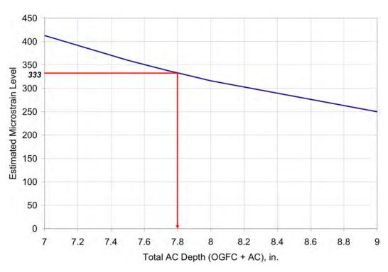
Figure 6 Approximate Relationship Between Strain and Thickness
