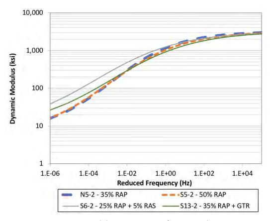
Figure 6 Dynamic Modulus Master Curves for Intermediate Layers
