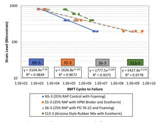
Figure 7 Bending Beam Fatigue Results for Bottom Layers
