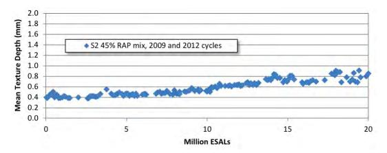
Figure 8 Macrotexture Results for 45% RAP Mix During 2009 and 2012 Cycles
