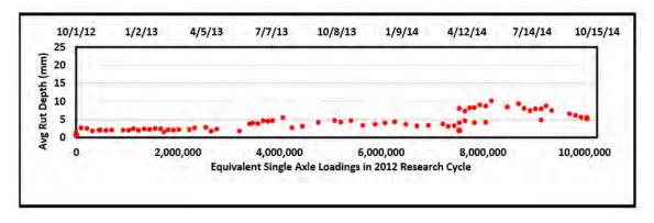
Figure 5 Rutting on Section N13 (OGI)
