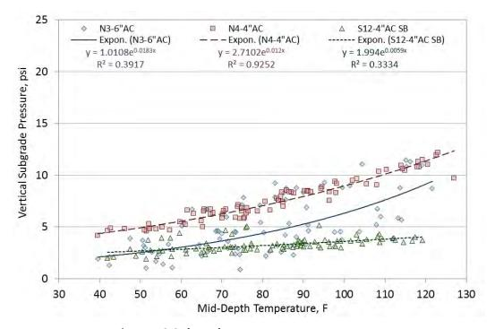
Figure 10 Subgrade Pressure vs. Temperature
