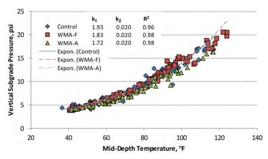
Figure 8 Subgrade Pressure Versus Temperature for WMA Sections and Control Section
