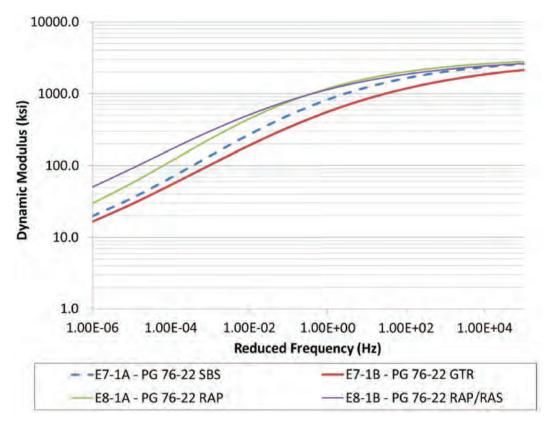
**Figure 1 FDOT Cracking Study Master Curves**
