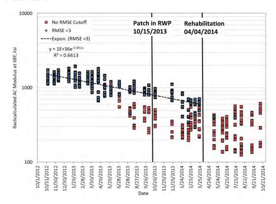
Figure 30 Section S6 (RAP/RAS) Backcalculated FWD Results
