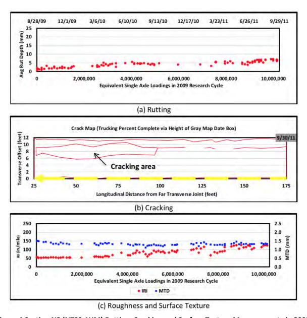
Figure 4 Section N2 (NTSS-1HM) Rutting, Cracking and Surface Texture Measurements in 2009
