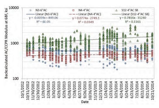
Figure 5 Backcalculated AC/CCPR Modulus at 68°F vs. Date
