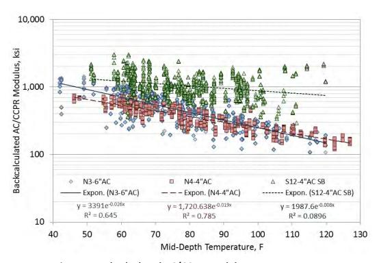
Figure 4 Backcalculated AC/CCPR Modulus vs. Temperature
