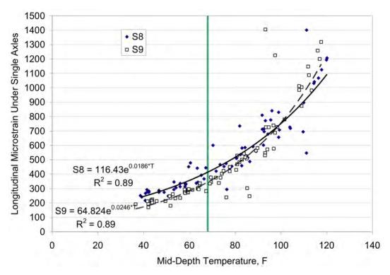
Figure 3 Strain Response of S8 (OGFC) and S9 (Control) Sections
