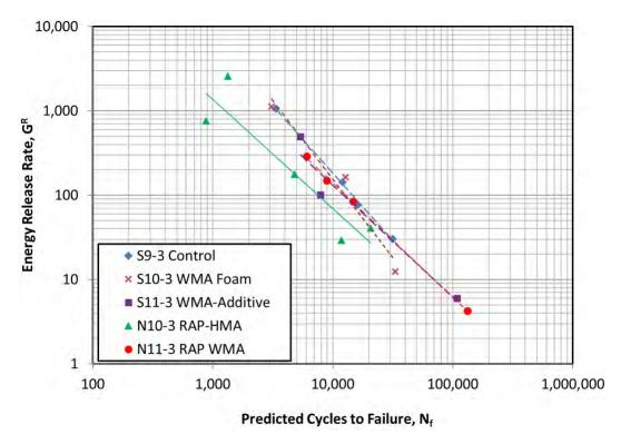
Figure 29 Predicted SVECD Cycles to Failure for Retested GE Base Layer Mixes
