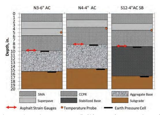
Figure 1 VDOT Experiment Average As-Built Thicknesses and Instrumentation Depth
