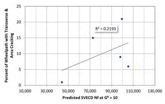
Figure 28 Relationship Between Predicted SVECD at G<sup>R</sup>=10 and Percent of Wheelpaths with Transverse and Area Cracking for GE
