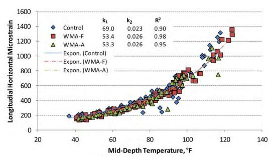
Figure 7 Longitudinal Strain Versus Temperature for WMA Sections and Control Section
