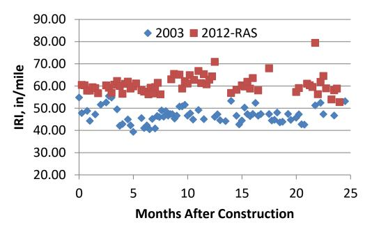
Figure 4 Roughness Measurements (IRI) for TNDOT Section S4
