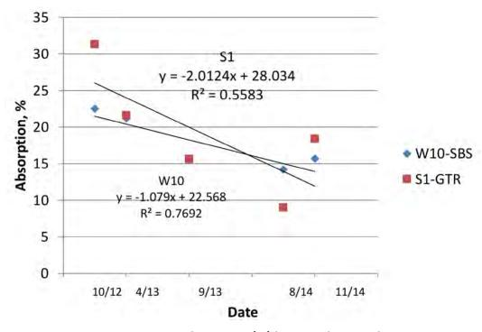
Figure 4 Noise Absorption (%) by Impedance Tube
