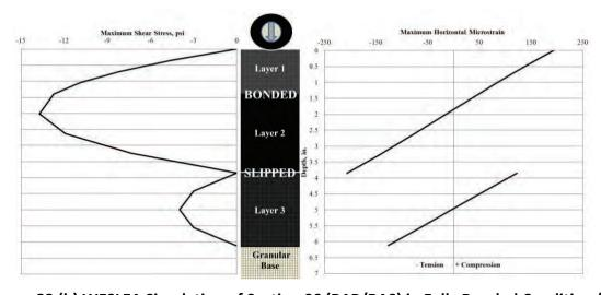
Figure 33 (b) WESLEA Simulation of Section S6 (RAP/RAS) in Fully Bonded Condition (1)
