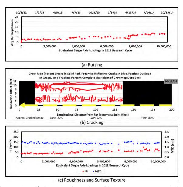
Figure 7 Section N2 (NTSS-1HM) Rutting, Cracking and Surface Texture Measurements in 2012
