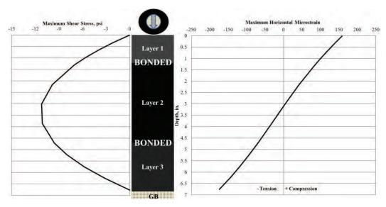
Figure 42 WESLEA Simulation of Section S13 (GTR) in Fully Bonded Condition (1)
