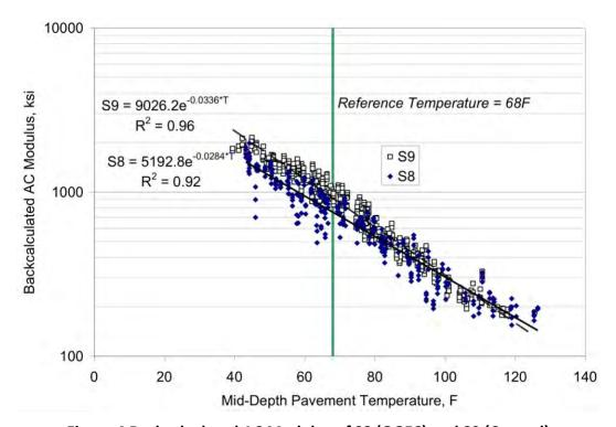
Figure 4 Backcalculated AC Modulus of S8 (OGFC) and S9 (Control)
