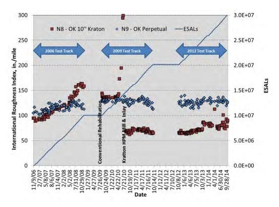
Figure 4 IRI Evaluation of Oklahoma Perpetual Pavement Sections
