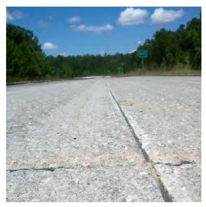
Figure 1 Deep Saw Cuts Simulating Pavement Cracks
