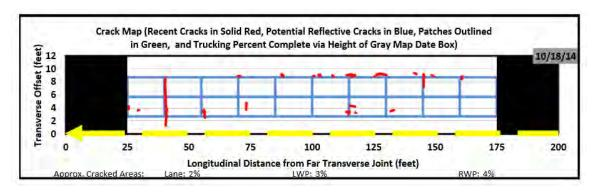
Figure 3 Crack Map of N13 (OGI Interlayer)
