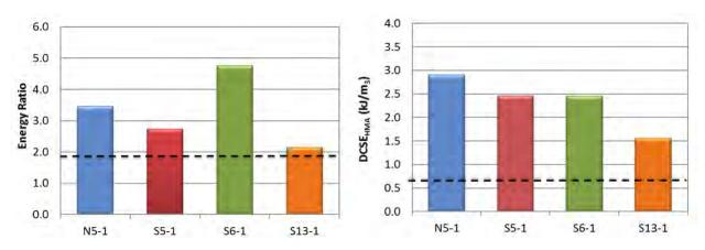
Figure 4 Energy Ratio Test Results for Green Group Surface Layers
