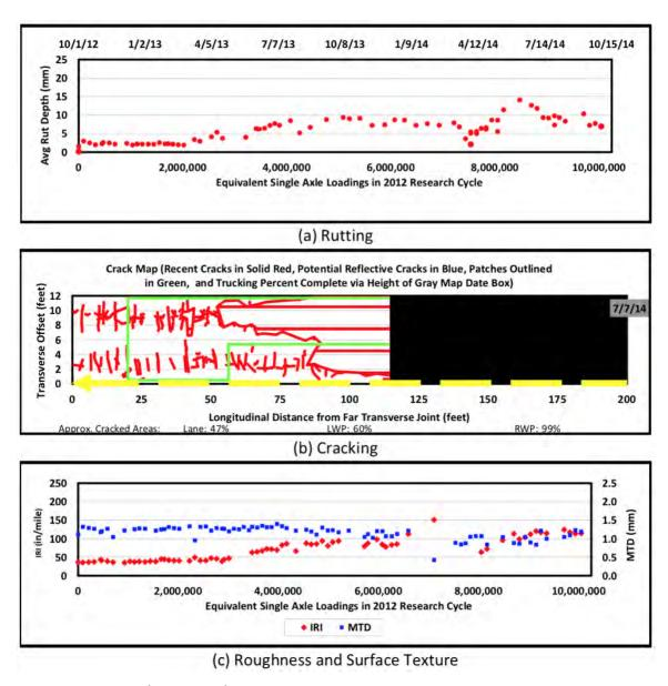
Figure 5 Section N1A (CRS-1HBC) Rutting, Cracking and Surface Texture Measurements in 2012
