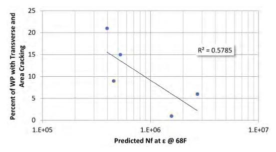
Figure 23 Relationship between Predicted BBF Nf at  $\epsilon_{68}$  and the Percent of Wheelpath with Transverse and Area Cracking for GE
