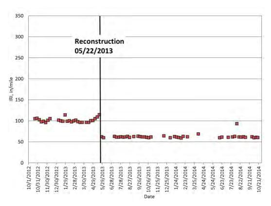
Figure 18 Section S5 (High RAP) Surface Performance
