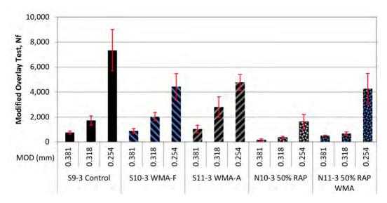
Figure 24 Results of Modified Overlay Test on GE Base Layer Mixes
