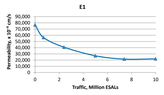
Figure 4 Loss of Permeability Reaches a Plateau in E1
