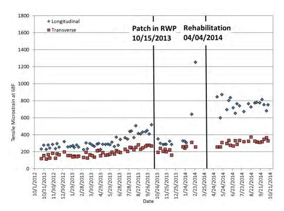
Figure 13 Section N5 (Standard RAP) Horizontal Strain
