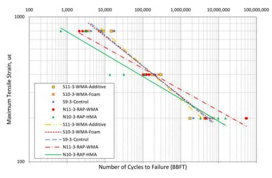
Figure 22 Bending Beam Fatigue Results for GE Base Layer Mixes
