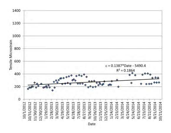
Figure 5 Temperature-Normalized Strain vs. Time
