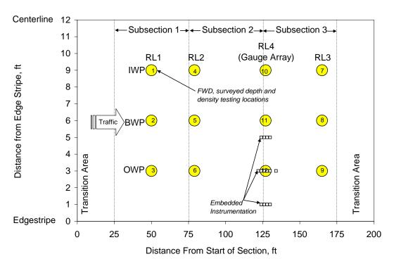
**Figure 6 Random Location and Instrumentation Schematic**
