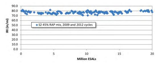
Figure 9 Roughness Results for 45% RAP Mix During 2009 and 2012 Cycles
