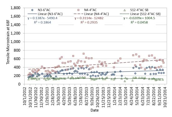
Figure 7 Tensile Strain at the Bottom of the CCPR Layer at 68°F vs. Time/Traffic
