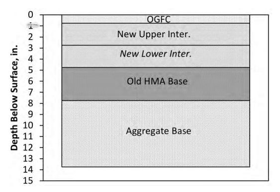
Figure 2 Pavement Cross-Section for N1 and N2 in 2009 and N1A, N1B, and N2 in 2012
