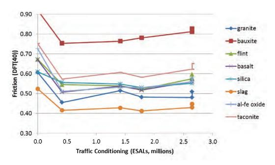
Figure 3. Left Wheel Path DFT(40) Fn Values After 2.6M ESALs
