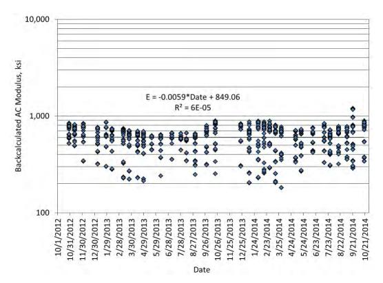
Figure 10 Temperature-Normalized AC Modulus vs. Time
