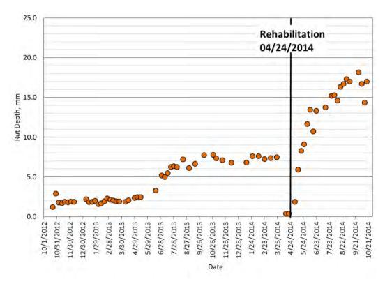
Figure 35 Section S13 (GTR) Rutting Performance
