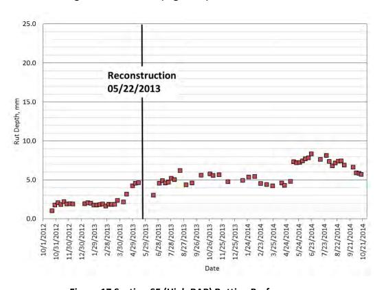
Figure 17 Section S5 (High RAP) Rutting Performance
