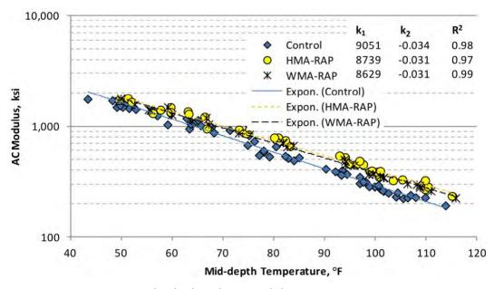
Figure 14 Backcalculated AC Modulus Versus Temperature
