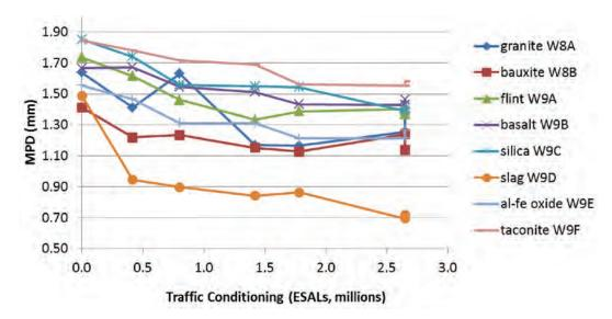
Figure 2 Left Wheel Path Surface Texture Values Measured by CTM
