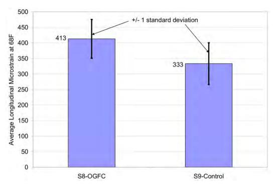
Figure 5 Strain Response Normalized to 68°F
