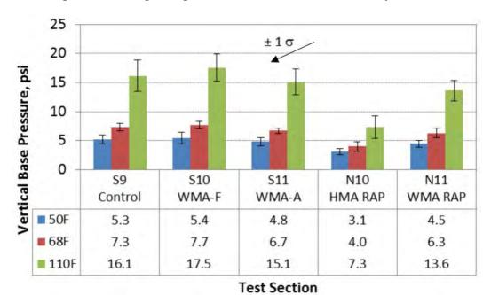
Figure 12 Average Vertical Pressures at Reference Temperatures
