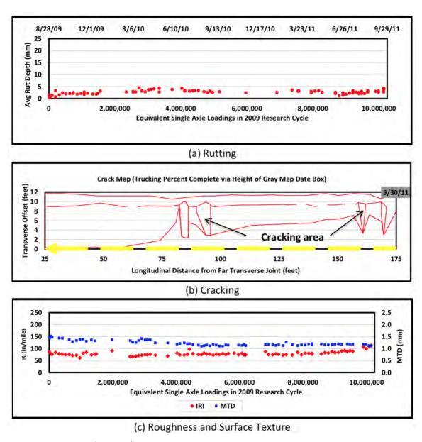
Figure 3 Section N1 (CRS-2P) Rutting, Cracking and Surface Texture Measurements in 2009
