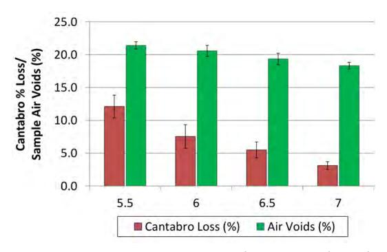
Figure 2 Section E9A 9.5 mm PFC Mix Design Cantabro Stone Loss and Air Voids
