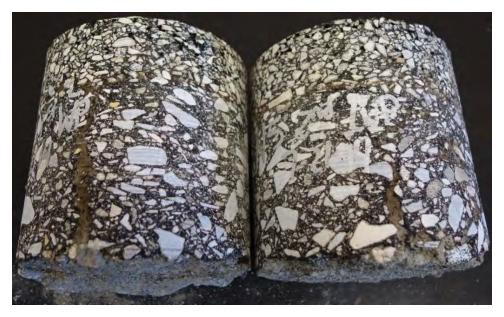
Figure 15 Section N5 (Standard RAP) Cores Showing Bottom-up Cracking
