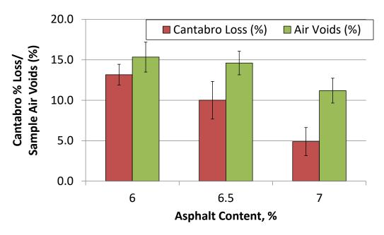
Figure 4 Cantabro Stone Loss for 12.5 mm NMAS PFC with 12% GTR
