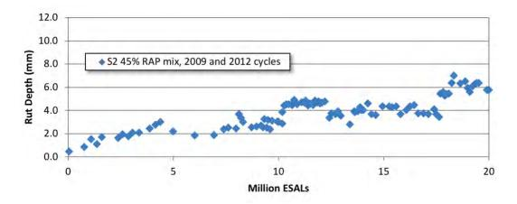
Figure 7 Rutting Results for 45% RAP Mix During 2009 and 2012 Cycles
