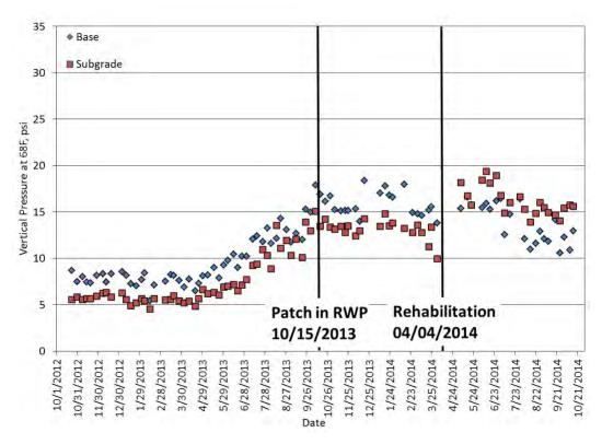
Figure 28 Section S6 (RAP/RAS) Vertical Pressure
