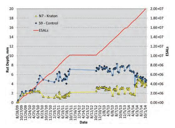
Figure 3 Kraton HPM Rutting Versus Time
