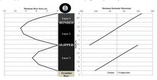
Figure 23 (b) WESLEA Simulation of Section S5 (High RAP) in Partial-Slip Condition (1)
