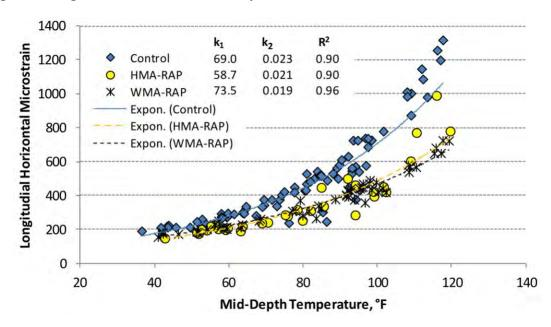
Figure 9 Longitudinal Strain Versus Temperature for 50% RAP Sections and Control Section
