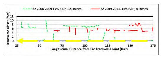
Figure 1 Crack Map for Section S2 at End of 2006 and 2009 Cycles
