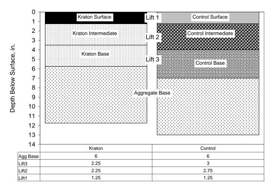
Figure 1 Cross-Section Design: Materials and Lift Thicknesses
