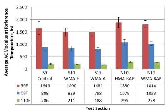
Figure 15 Average AC Modulus at Reference Temperature
