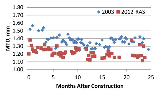
Figure 2 Comparison of MTD for TNDOT Section S4
