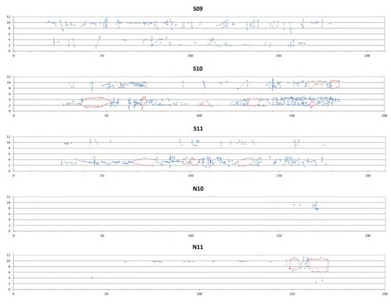
Figure 18 Crack Maps for GE Sections as of December 16, 2013
