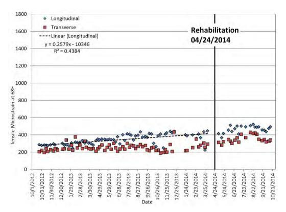
Figure 38 Section S13 (GTR) Horizontal Strain
