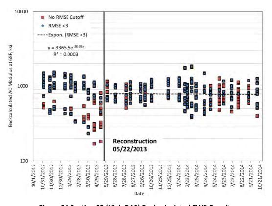
Figure 21 Section S5 (High RAP) Backcalculated FWD Results
