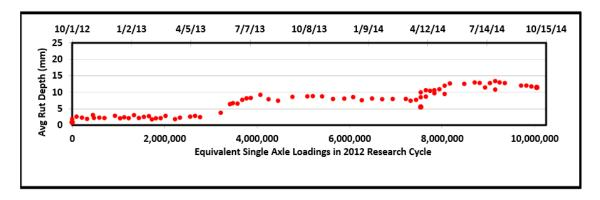
Figure 4 Rutting on Section N12 (Surface Treatment Interlayer)
