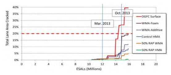
**Figure 17 Cracking Performance of Group Experiment Test Sections**
