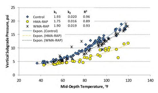
Figure 10 Subgrade Pressure Versus Temperature
