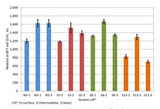
Figure 5 Dynamic Modulus Comparison at 68°F and 10 Hz
