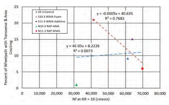
Figure 30 Relationship between Retested SVECD N<sub>f</sub> at G<sup>R</sup>=10 and Percent of Wheelpaths with Transverse and Area Cracking
