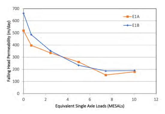
Figure 4 Field Permeability Measurements for Sections E1A and E1B
