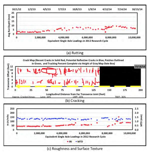
Figure 6 Section N1B (NT-HAP) Rutting, Cracking and Surface Texture Measurements in 2012
