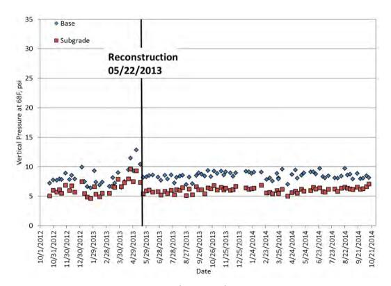
Figure 19 Section S5 (High RAP) Vertical Pressure
