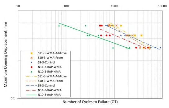
Figure 25 OT Results at Three MOD Levels for GE Base Layer Mixes
