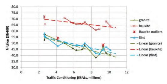
Figure 5 Left Wheel Path Field Skid Trailer Testing Summary
