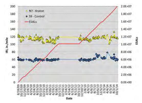
Figure 2 Kraton HPM Roughness Versus Time
