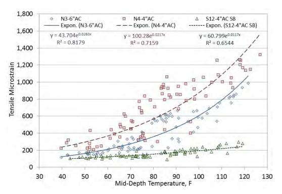
Figure 6 Tensile Strain at the Bottom of the CCPR Layer vs. Temperature
