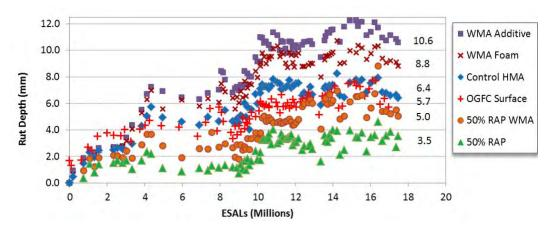
Figure 16 Rutting Performance of Group Experiment Test Sections
