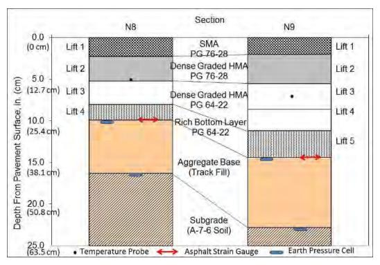
Figure 1 Structural Cross Sections and Instrumentation (1)
