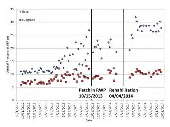
Figure 12 Section N5 (Standard RAP) Vertical Pressure
