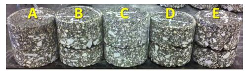
Figure 22 (a) Cores Taken from Section S5 (High RAP) in April 2013
