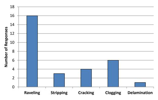
Figure 2 Type of Distress Observed in PFC Pavements
