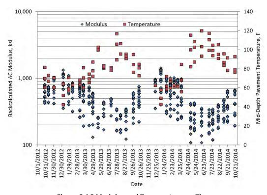
Figure 8 AC Modulus and Temperature vs. Time
