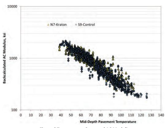
**Figure 6 Temperature Corrected AC Moduli**
