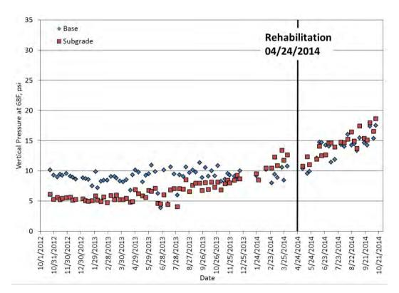
Figure 37 Section S13 (GTR) Vertical Pressure
