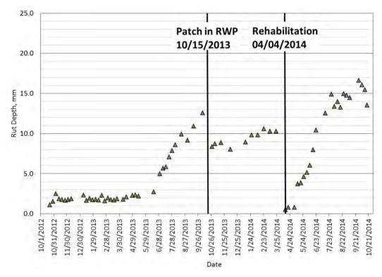
Figure 26 Section S6 (RAP/RAS) Rutting Performance
