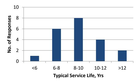
**Figure 1 Typical Performance Life of PFC Mixtures**
