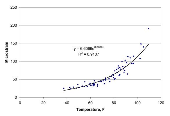
Figure 5.10. Strain-Temperature Relationship for Steer Axles in N9 (29)
