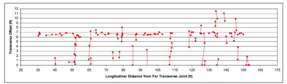
Figure 7.2. Crack Map for Original Section S2 Near End of the 2003 Research Cycle
