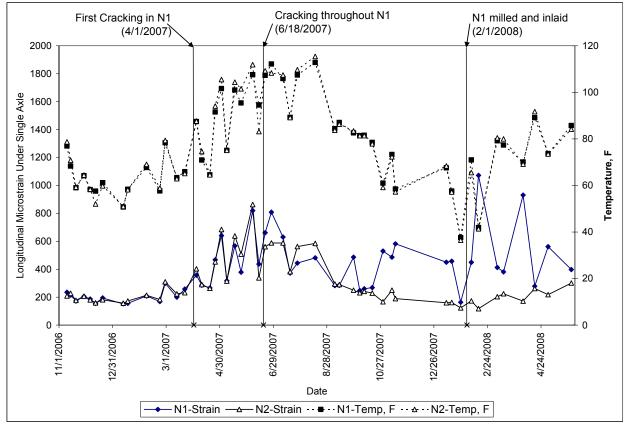
Figure 3.2. Measured Strain and Temperature versus Date (9)
