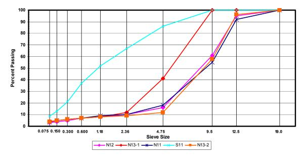
Figure 3.11. Aggregate Gradations of the Sections
