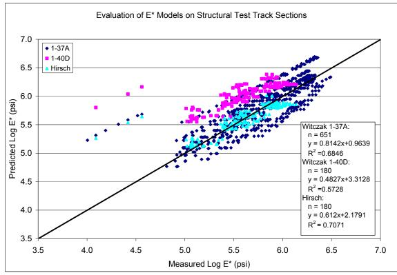
Figure 6.12. Comparison of Predicted E\* Values to Measured E\* Values by Model
