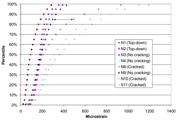
Figure 5.11. Cumulative Distribution of Strains for 2006 Structural Sections (29)
