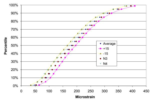
Figure 5.13. Average Strain Distribution with Confidence Bands (29)
