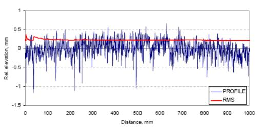
Figure 3.9. RMS Filter Applied to ULIP Surface Profile (15)
