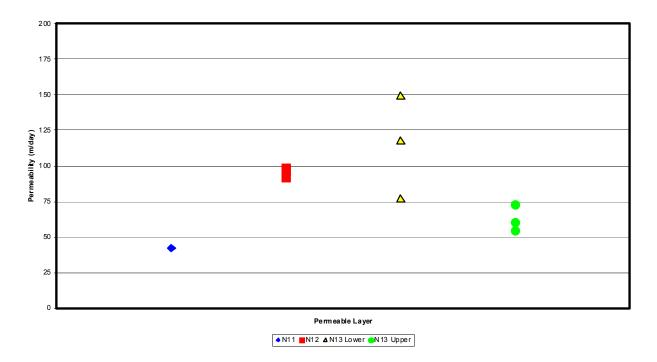
Figure 3.15. Laboratory Permeability Measurements from Cut Cores (14)
