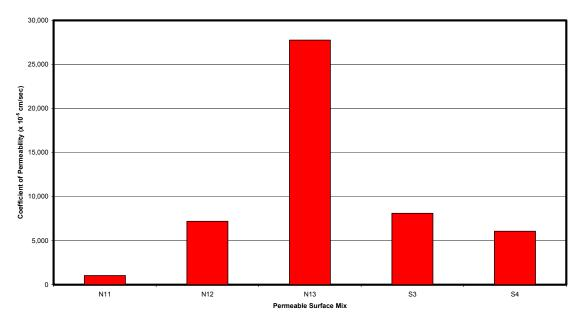
Figure 7.4. Coefficient of Permeability in Drainable Surfaces Using Field Permeameter.
