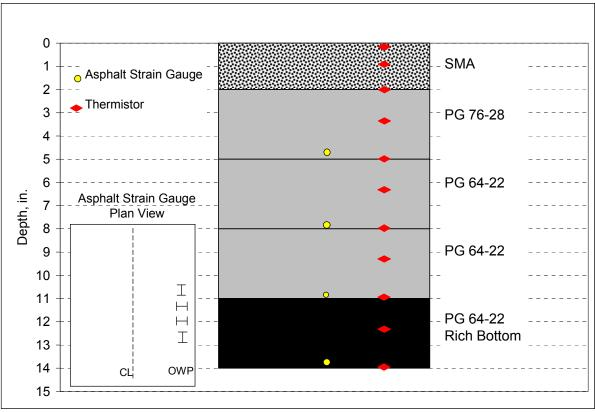
Figure 4.2. N9 Supplemental Instrumentation (2)
