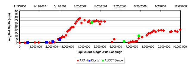
Figure 3.29. Rutting Progression in Section S8B Showing Replacement Mix
