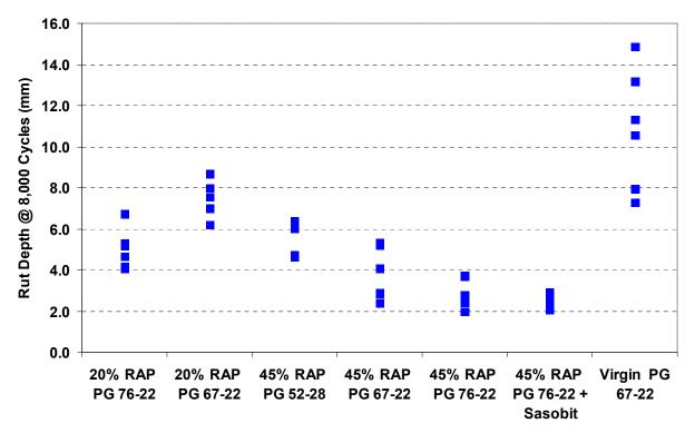
Figure 3.4. Rut Depths from APA Testing (13)
