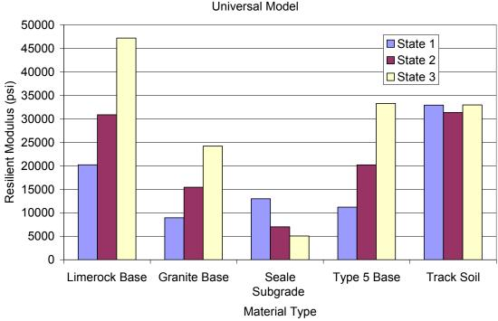
Figure 6.1. Unbound Material Moduli at Representative Stress-States – Universal Model (27)
