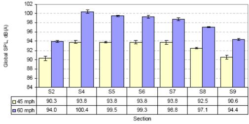
Figure 3.7. Summary of Global Sound Pressure Levels at 45 and 60 mph (15)
