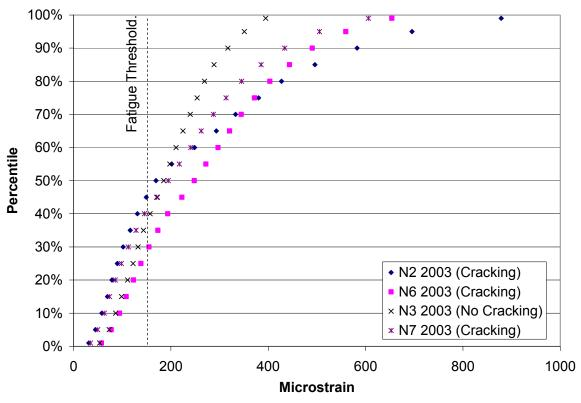
Figure 6.13. Endurance Limits for PG 67-22 Mix (29)
