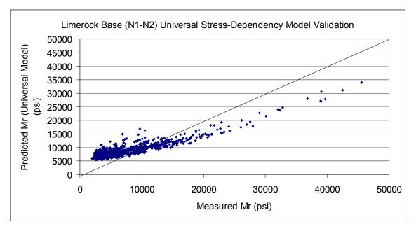
Figure 6.7. Limerock Base Universal Stress-Sensitivity Model Validation (27)
