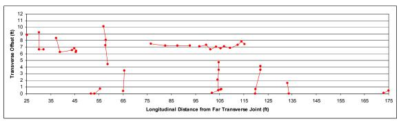
Figure 7.3. Cracking Exhibited after 10 million ESALs in Section S2
