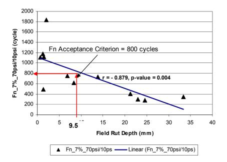
Figure 3.28. Correlation Between Flow Number and Field Rutting Performance
