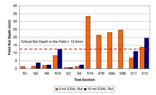
Figure 3.26. Comparison of Field Rut Depths after 5 and 10 million ESALs
