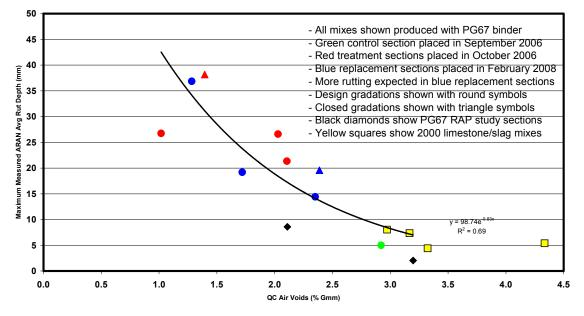
Figure 3.30. Relationship Between Rutting and QC Air Voids
