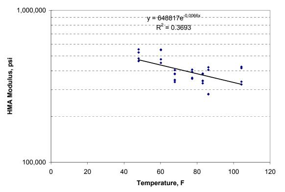
Figure 5.3. HMA and Temperature Relationship for S10 (29)
