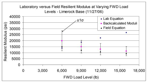
Figure 6.9. Laboratory versus Field Resilient Moduli Comparison (Limerock Base Material, FWD Testing on 11/27/06) (27)
