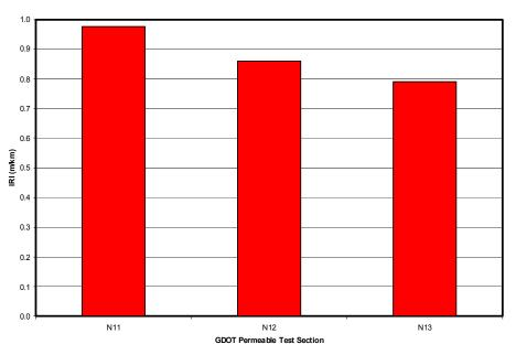
Figure 3.12. Post-Construction Smoothness Comparison (14)
