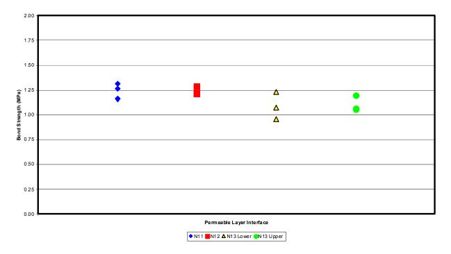
Figure 3.14. Interlayer Bond Strength Measurements from Mat Cores (14)
