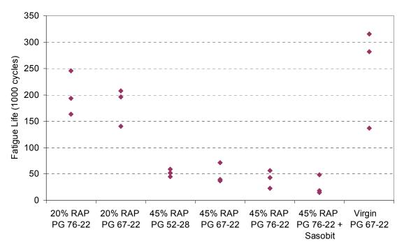
Figure 3.6. Plot of Beam Fatigue Test Results for the RAP Experimental Sections (13)
