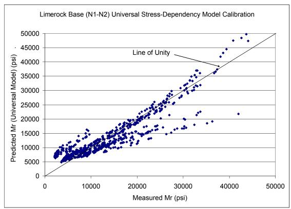
Figure 6.6. Limerock Base Material Universal Model Calibration Data (27)
