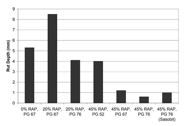
Figure 3.3. Field Rut Depths after 10 Million ESALs for the RAP Experimental Sections
