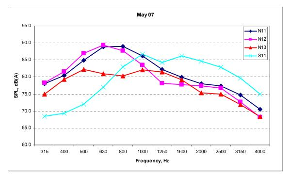
Figure 3.21. Noise Spectra – May-07 Measurements
