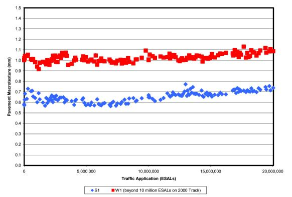
Figure 7.5. Increase in Macrotexture of High LA Abrasion Loss SMA Surface
