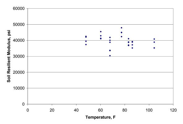
Figure 5.4. Soil Resilient Modulus and Temperature Relationship for S10 (29)
