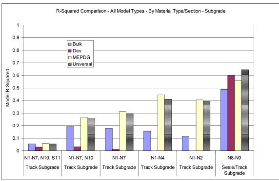
Figure 6.5. Model R-Squared Summary (Subgrade Layer, by Material) (27)
