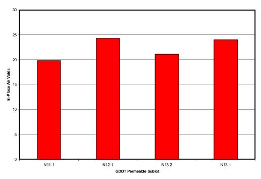
Figure 3.13. Post-Construction Air Voids for all Porous Surface Lift Sublots (1 = Upper Lift, 2 = Lower Lift) (<u>14</u>)
