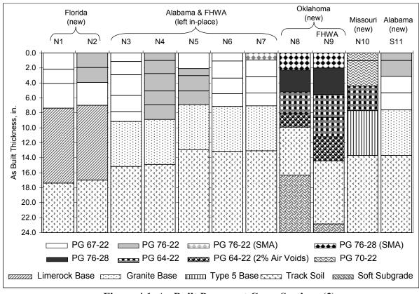
Figure 4.1. As-Built Pavement Cross Sections (2)
