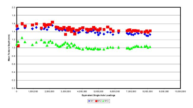
Figure 3.17. Macrotexture Measurements as a Function of Truck Traffic (14)
