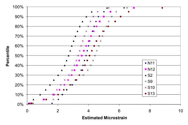
Figure 5.5. Cumulative Distributions of Strain for 2000 Test Track (29)
