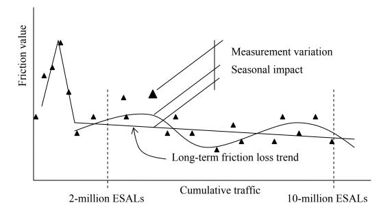
Figure 3.10. Generic HMA Surface Friction Performance Curve
