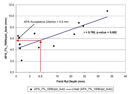
Figure 3.27. Correlation between APA Rut Depths and Field Rutting Performance
