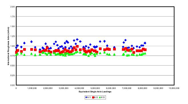
Figure 3.16. Roughness Measurements as a Function of Truck Traffic (14)
