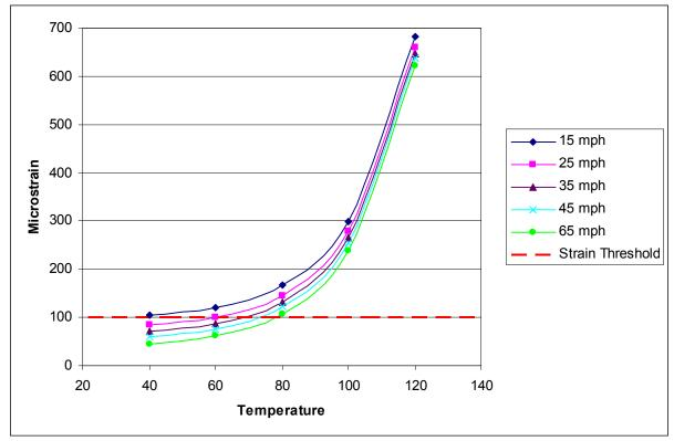
Figure 5.1. Predicted Strain by Temperature for a Single Axle
