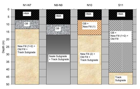
Figure 6.3. Final Selected Backcalculation Cross-Sections (27)
