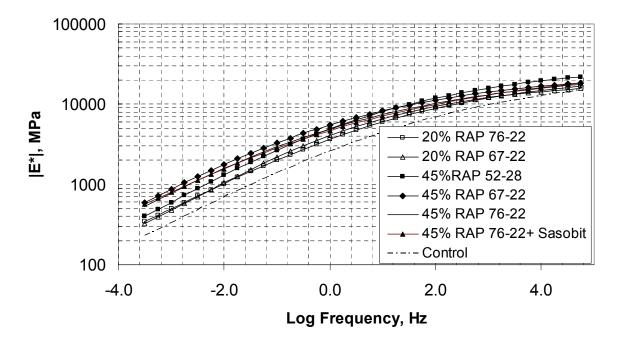
Figure 3.5. Master Curves of Dynamic Moduli for the RAP Experimental Sections (13)
