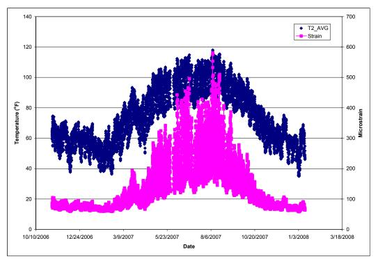
Figure 5.2. Measured Strain and Mid-Depth Temperatures for the N9 Test Section (28)
