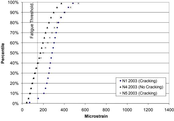
Figure 6.14. Endurance Limits for PG 76-22 Mix (29)
