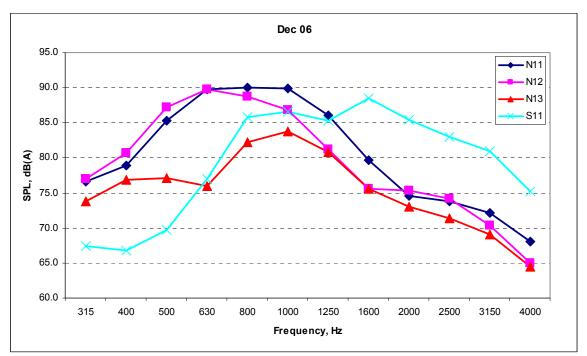
Figure 3.19. Noise Spectra – Dec-06 Measurements
