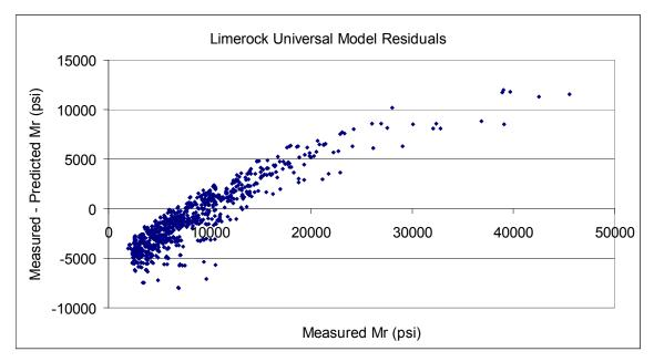
Figure 6.8. Limerock Base Universal Stress-Sensitivity Model Residuals (27)
