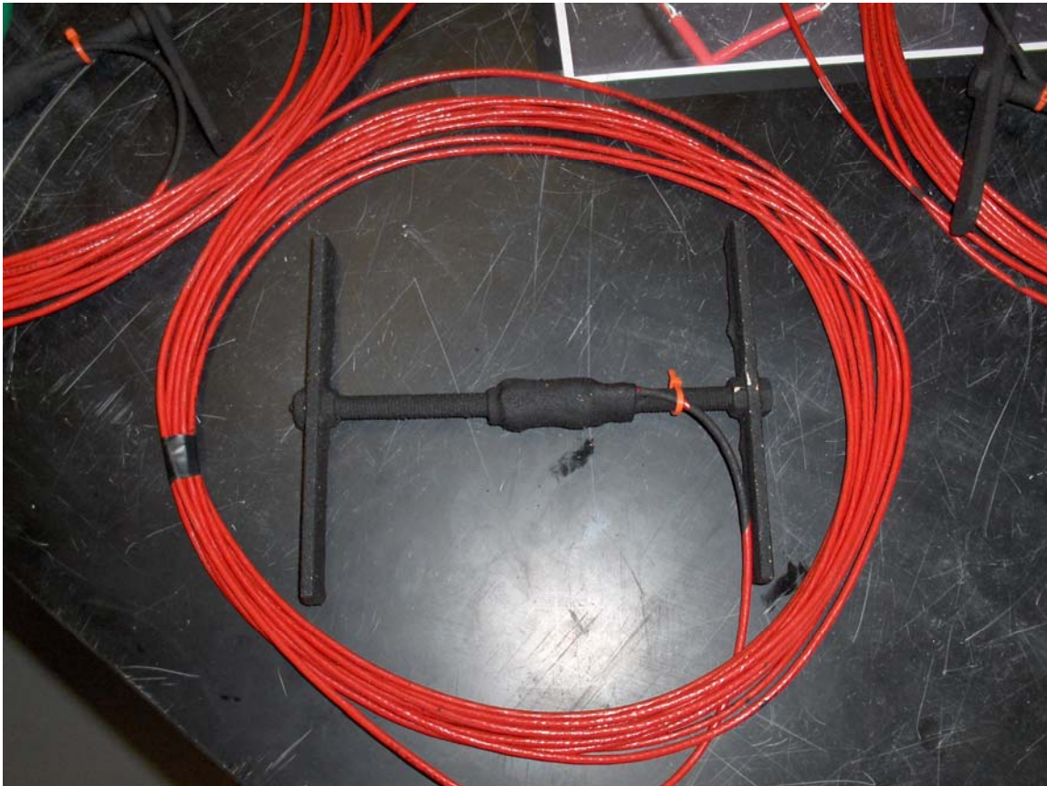
Figure 1. CTL ASG-152 Strain Gauge
