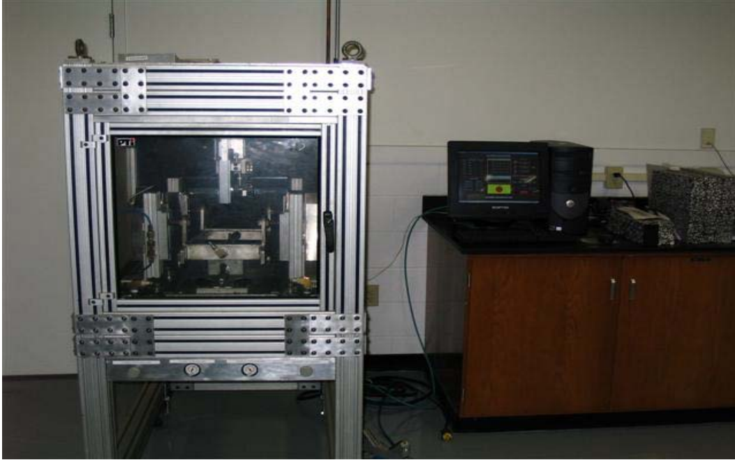
Figure 1 Mix Verification Tester
