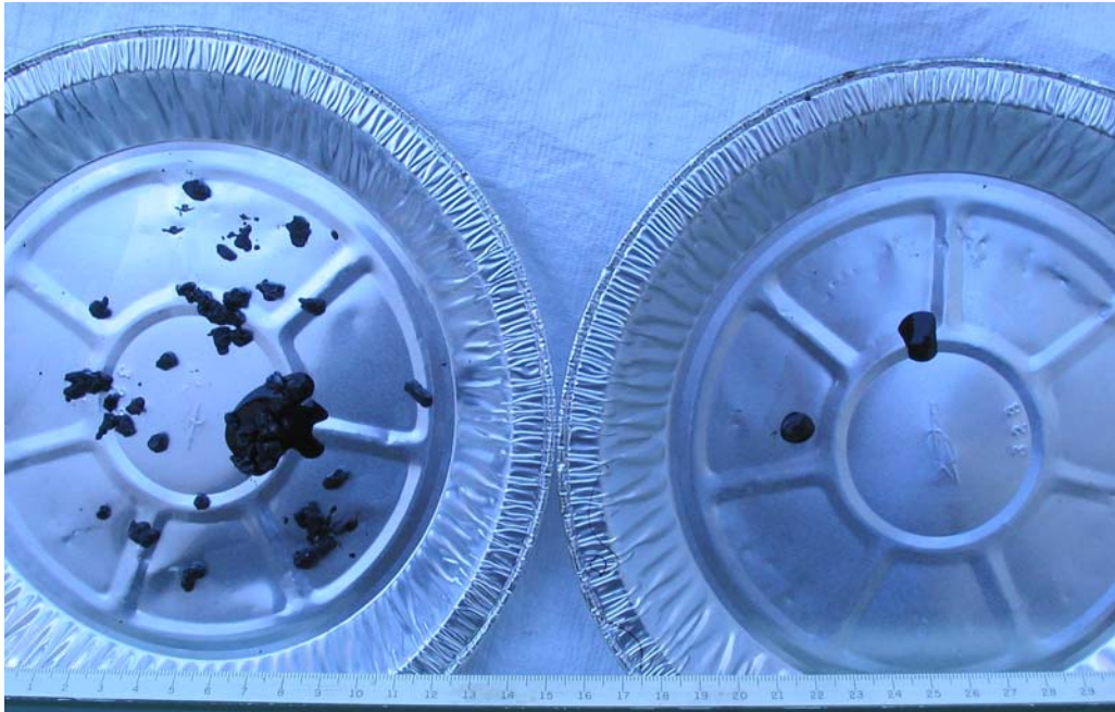
Figure 12. Sample Draindown Test Results (Granite @ 7.5% AC)
