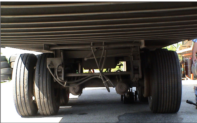
Figure 1 A standard dual-tire configuration (left) and a wide-base single tire (right).
