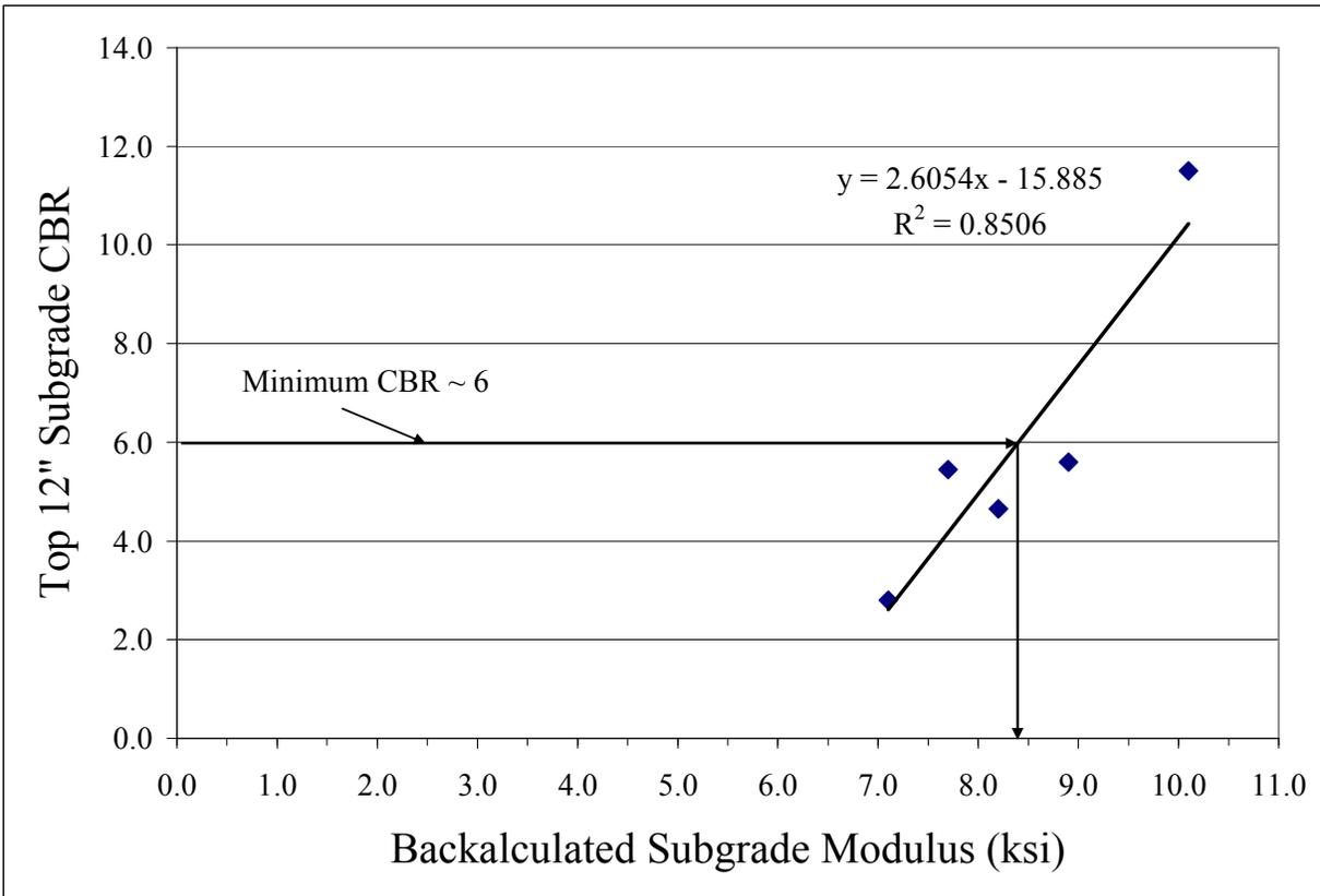
**Figure 3.5, Subgrade CBR vs Modulus for Texas FM 1155**
