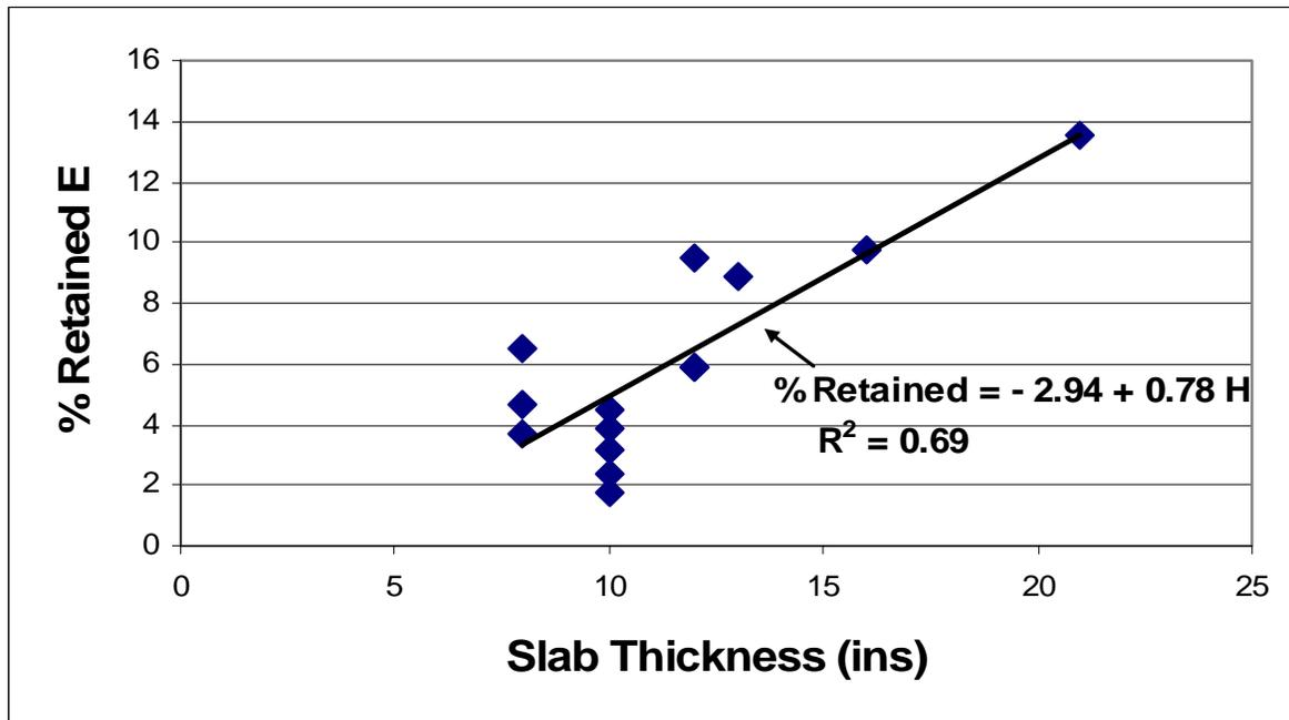
**Figure 4.9, “Retained Modulus” Percent versus Slab Thickness**
