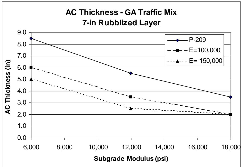
**Figure 4.12, HMA (AC) Design Overlay Thicknesses for Light Traffic (GA) Mix**
