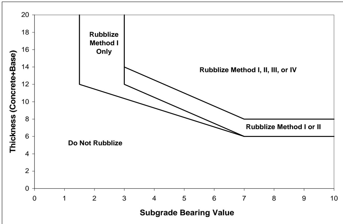
Figure 3.2, Illinois DOT Rubblization Selection Chart [Heckel, 2002].
