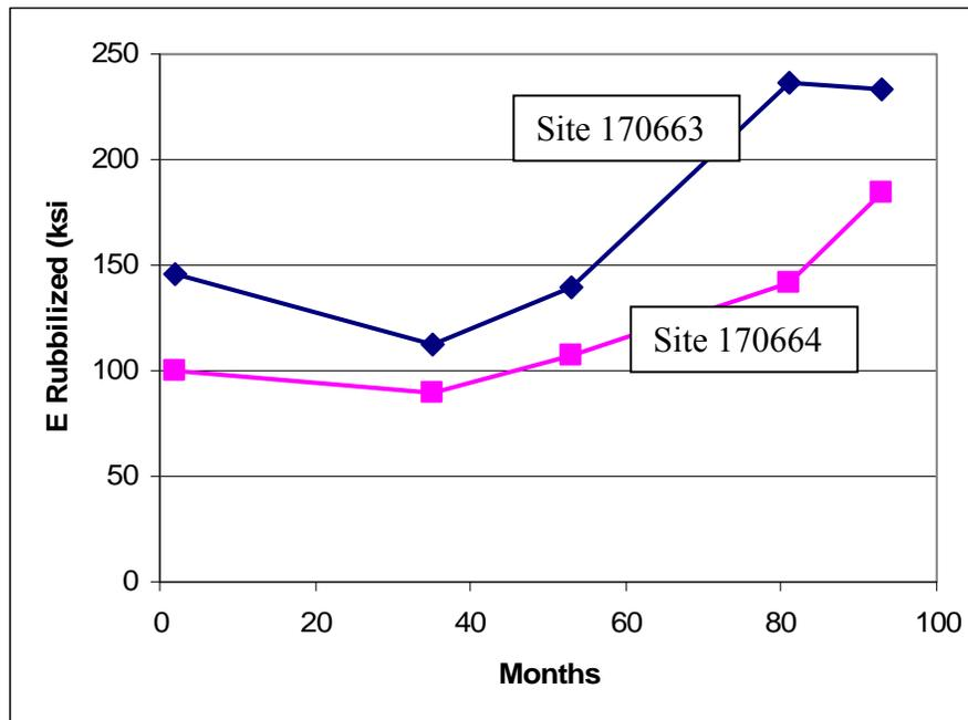
**Figure 4.6, Plot of Rubblized Layer Moduli versus Time from Illinois LTPP Sites**
