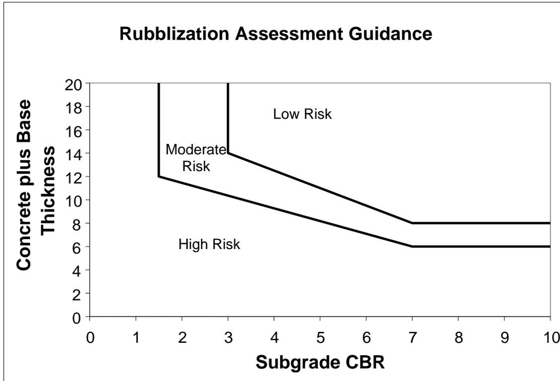
**Figure 3.8, Proposed Rubblization Assessment Chart for Airfields with Slabs < 9 Inches**
