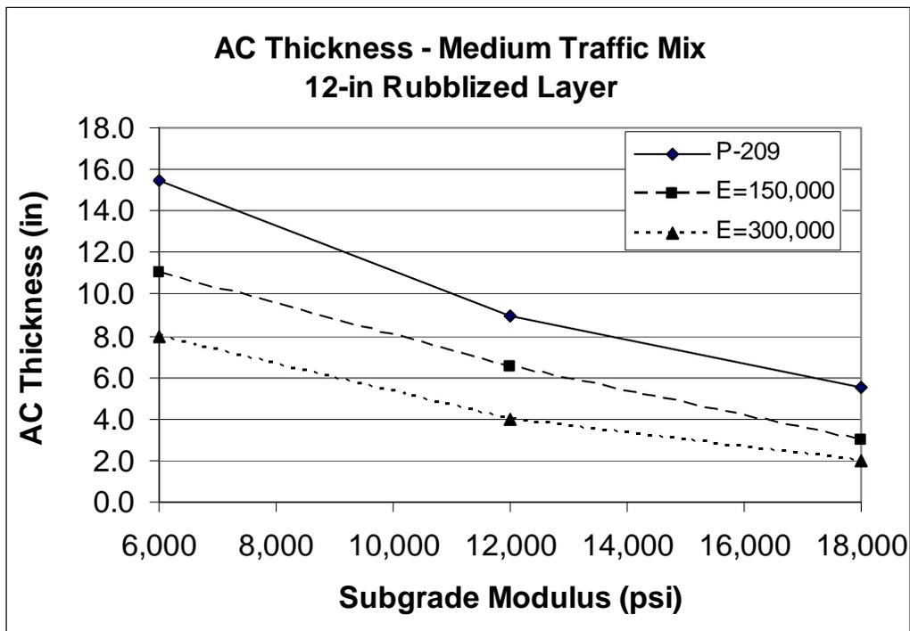
Figure 4.11, HMA (AC) Design Overlay Thicknesses for Medium Traffic Mix
