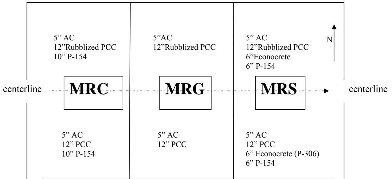
**Figure 2.4, Layout of Test Sections at NAPTF [Garg, 2006]**
