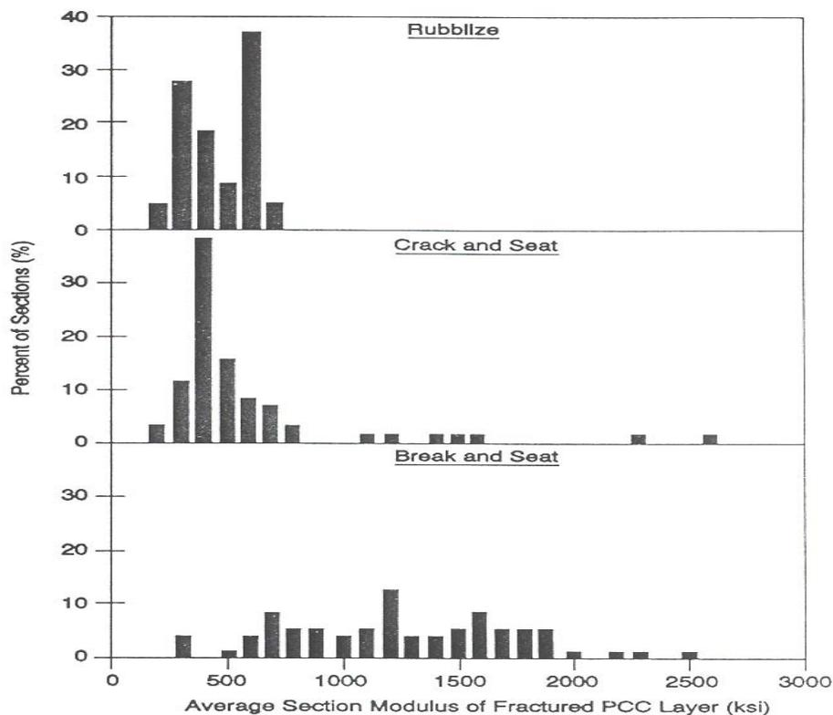
**Figure 4.1, Frequency Distribution of In-situ PCC Moduli after Fracture [Witczak, 1992]**
