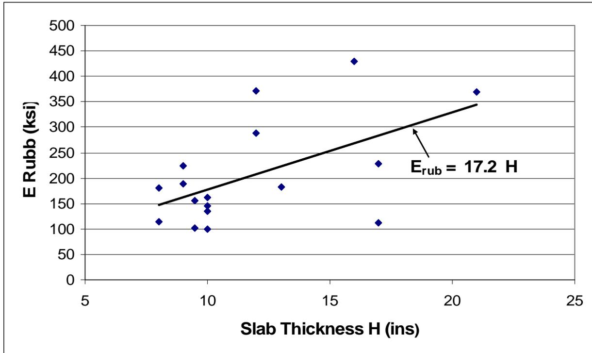
**Figure 4.8, Average Initial Moduli versus Slab Thickness for All Sections Discussed**
