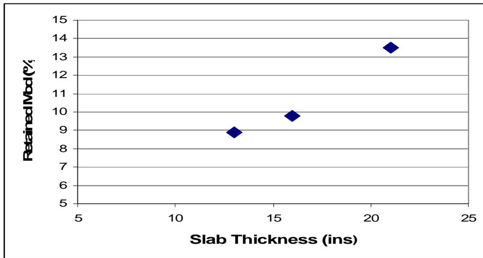
**Figure 4.2, Retained Modulus versus Slab Thickness at Selfridge ANGB**
