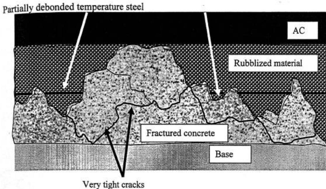
**Figure 2.1, Schematic of “Crushed” and “Fractured” Layers [Baladi et al, 2002]**
