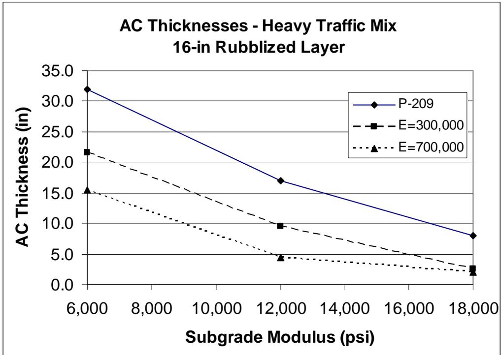
Figure 4.10, HMA (AC) Design Overlay Thicknesses for Heavy Traffic Mix
