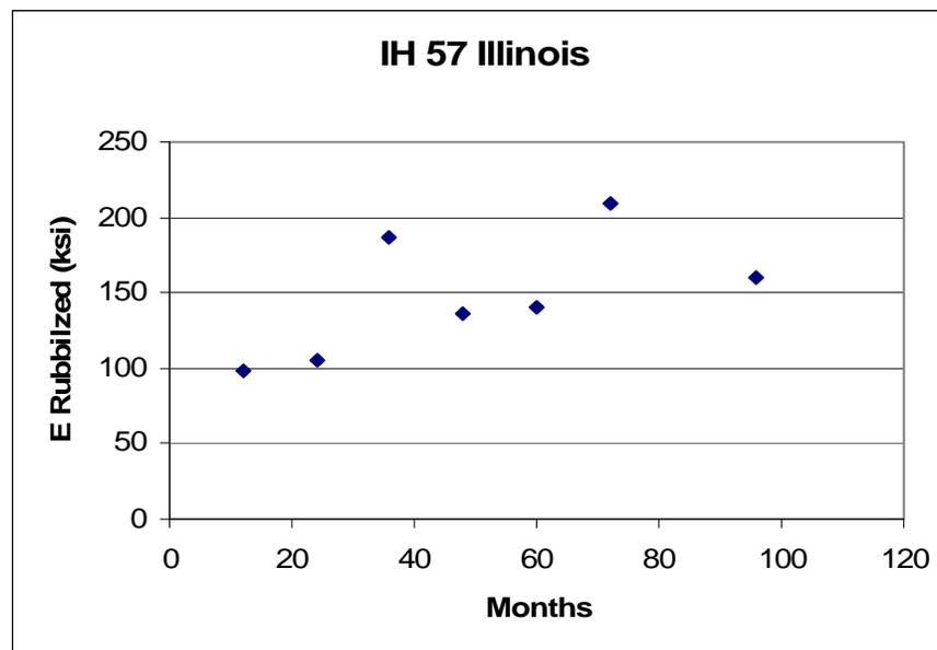
**Figure 4.3, Change in Rubblized Modulus with Time, I-57 Illinois**
