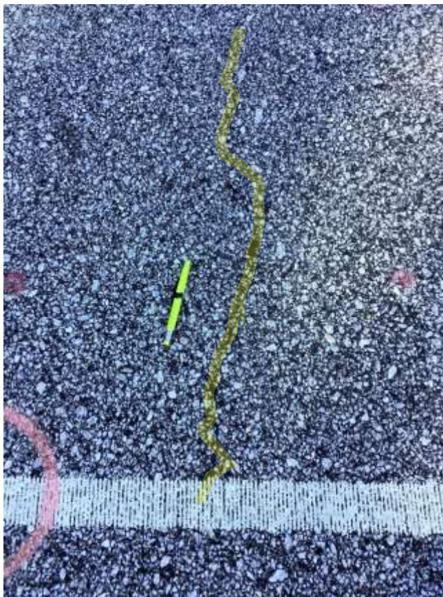
FIGURE 3 Longitudinal crack at edge of outside wheelpath in S9 at end of first test cycle.
