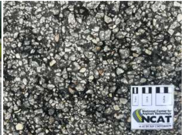
E5B (92.0% of G_{mm} ) representative cracking
