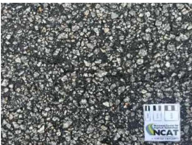
E6A (87.8% of G_{mm} ) representative cracking
