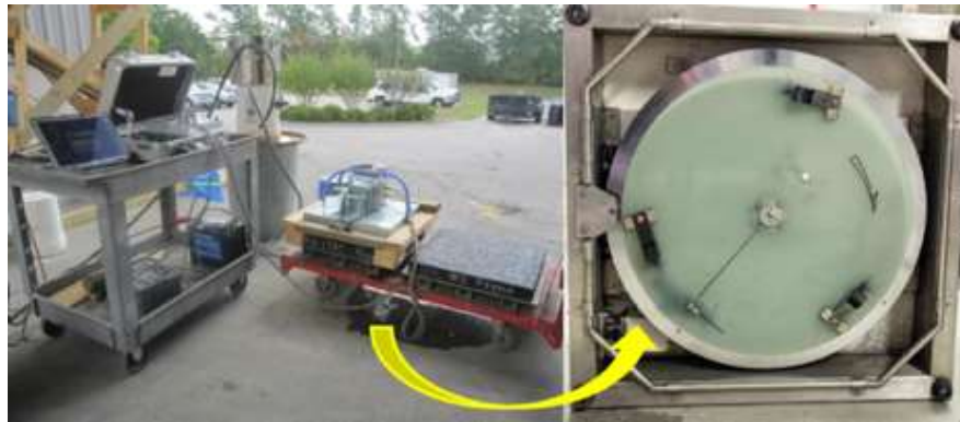
FIGURE 9 Dynamic friction tester (DFT).
