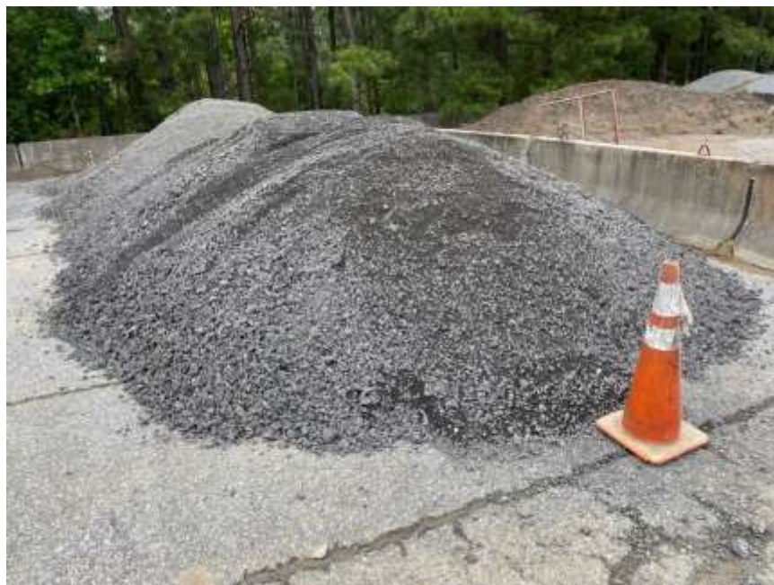
FIGURE 3 Stockpiled reclaimed CCPR millings.
