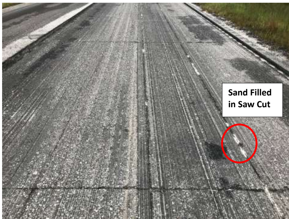
FIGURE 1 Deep saw cuts to simulate pavement cracks.
