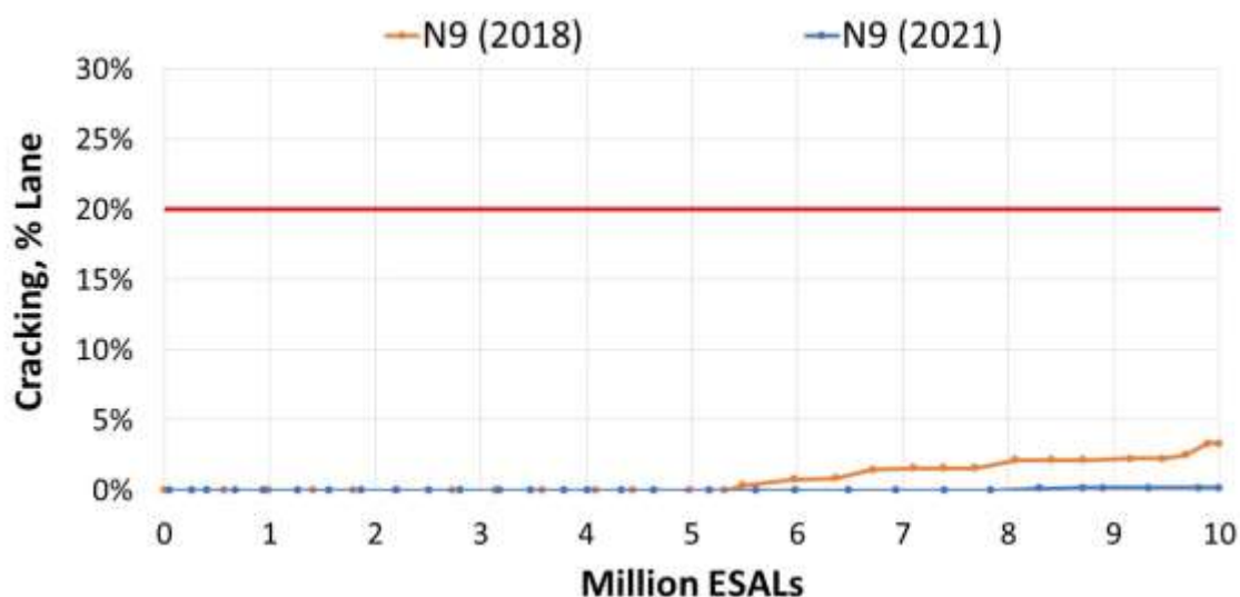
FIGURE 21 Cracking data of Section N9 (2018 and 2021 test cycles).
