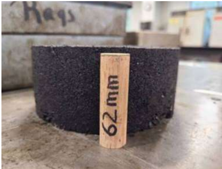
FIGURE 15 Typical expansion with RTR specimens.
