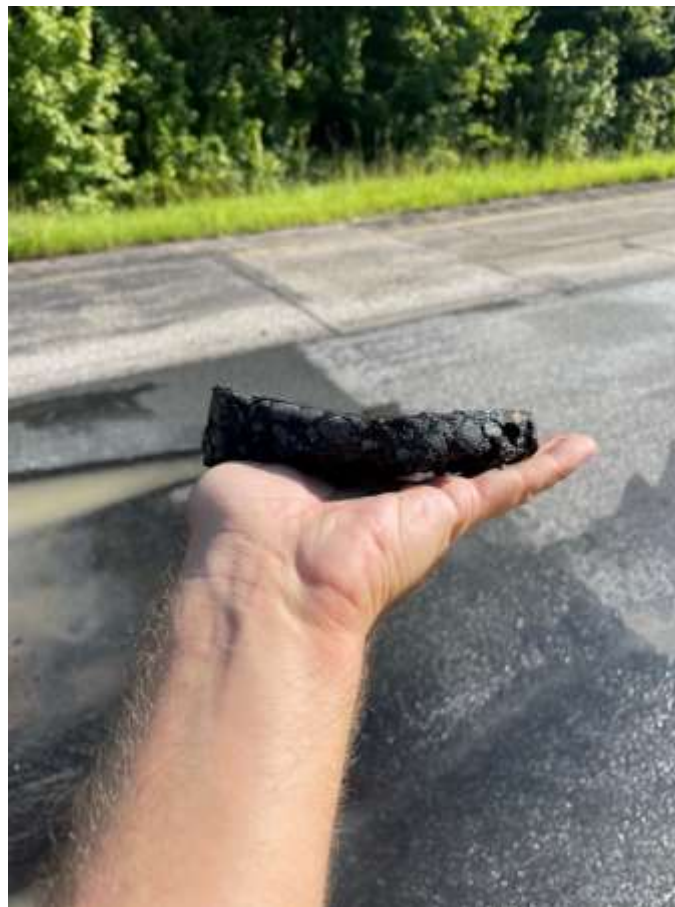
FIGURE 11 A core sample of the SMA layer in the transition zone at the end of the Section.
