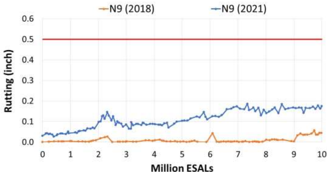
FIGURE 19 Field rutting data of Section N9 (2018 and 2021 test cycles).
