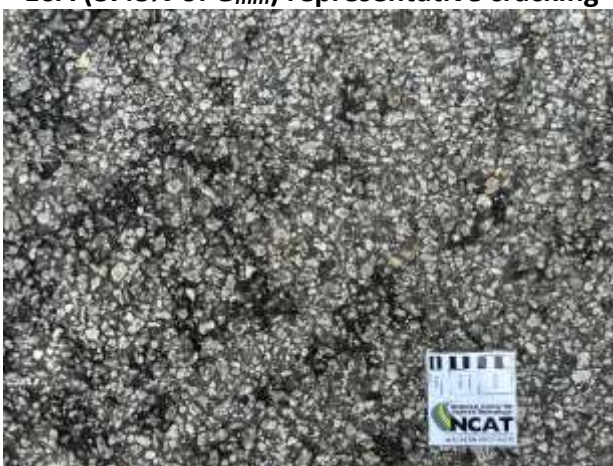
E6B (89.7% of G_{mm} ) representative cracking
