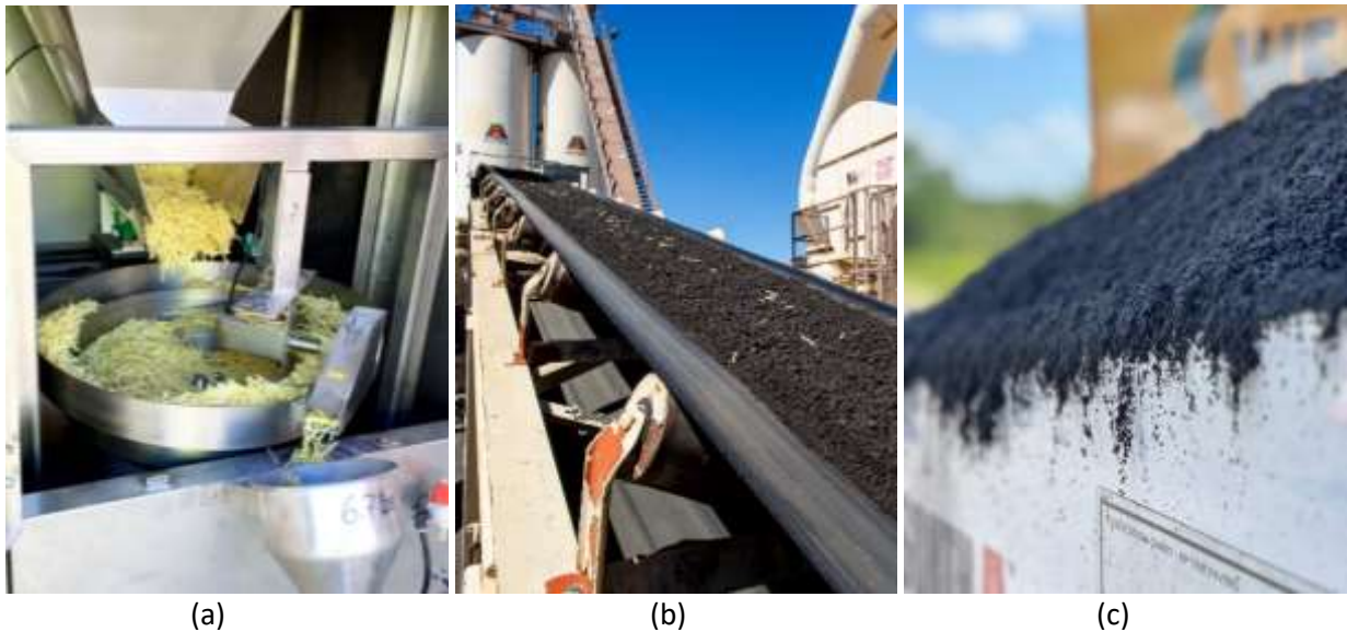
FIGURE 2 Synthetic fiber used in the AG experiment: (a) Fiber stands in dosing equipment, (b) Fiber strands dosed on RAP belt to mixing drum, (c) Individual fibers dispersed into the mix.
