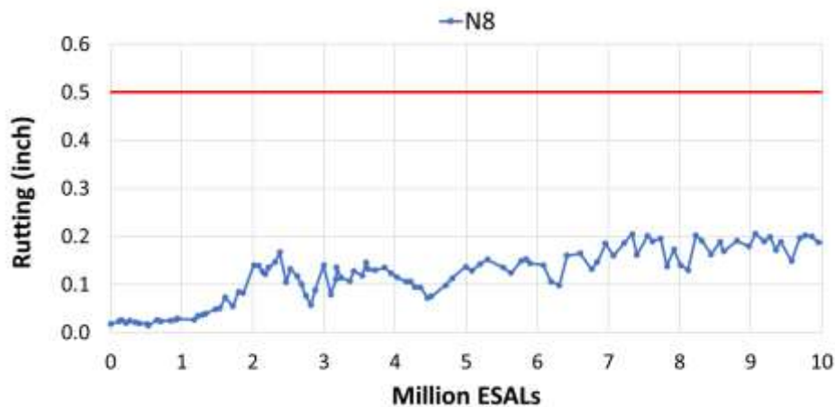
FIGURE 12 Field rutting data of Section N8.
