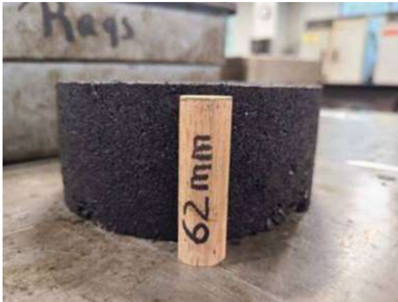
FIGURE 15 Typical expansion with RTR specimens.
