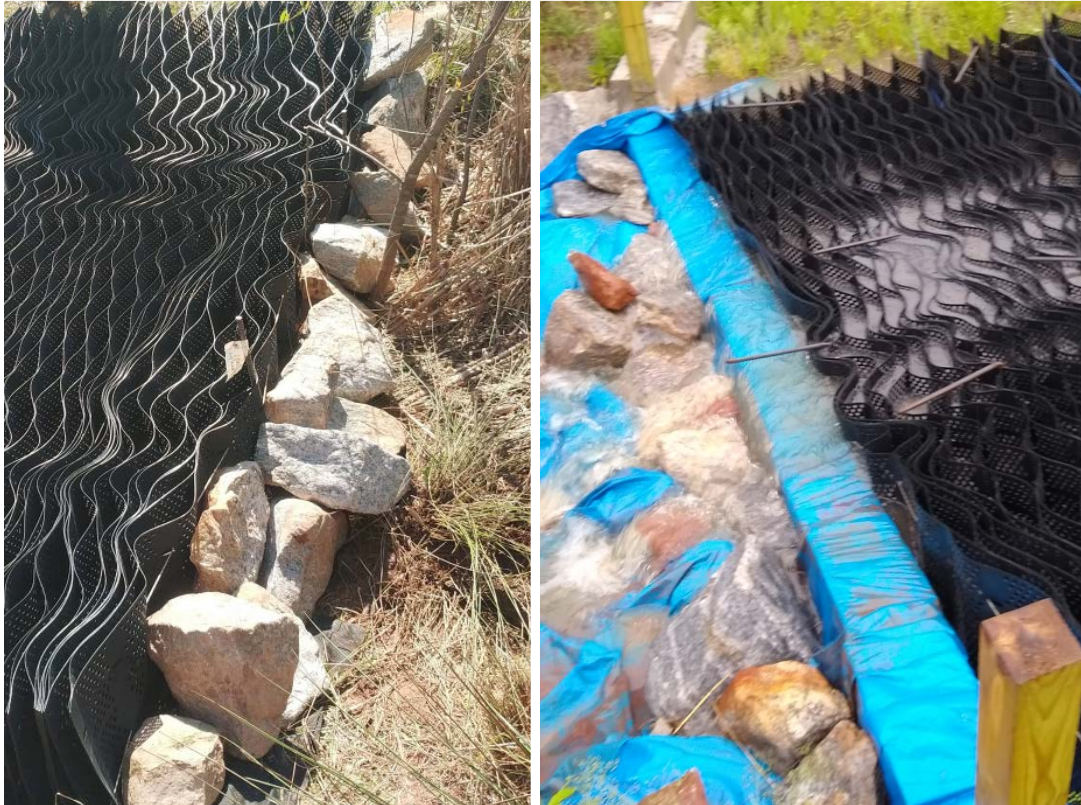
Figure 4 – Details of the upstream (Left) and downstream (Right) ends of the experimental apparatus, including the weir locations at the downstream end to gauge flow depth and calculate flow rates over the weir.
