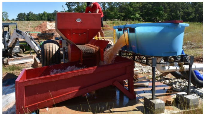
Flow and sediment introduction apparatus
