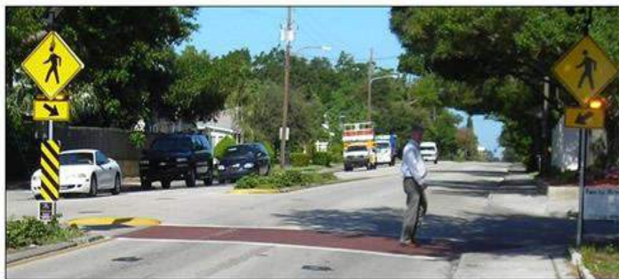
Figure A- 8. RRFB system (Pechoux et al. 2009).
