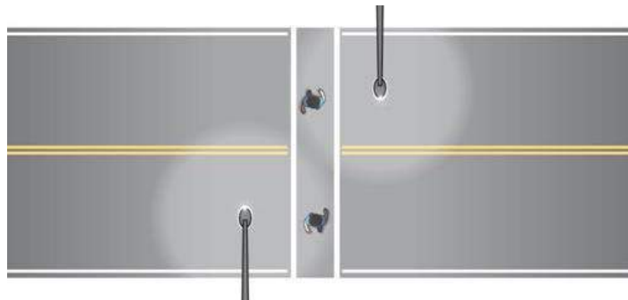
Figure A- 12. Midblock crosswalk lighting layout (Gibbons et al. 2008).
