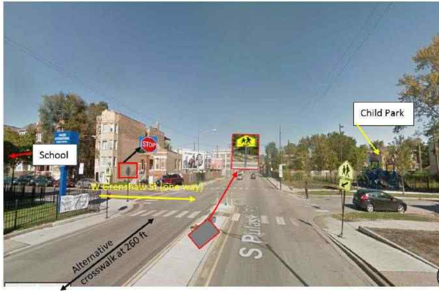
Figure E-65. Existing stop control on minor street- with median at the intersection of S. Pulaski Rd. and W. Grenshaw St.
