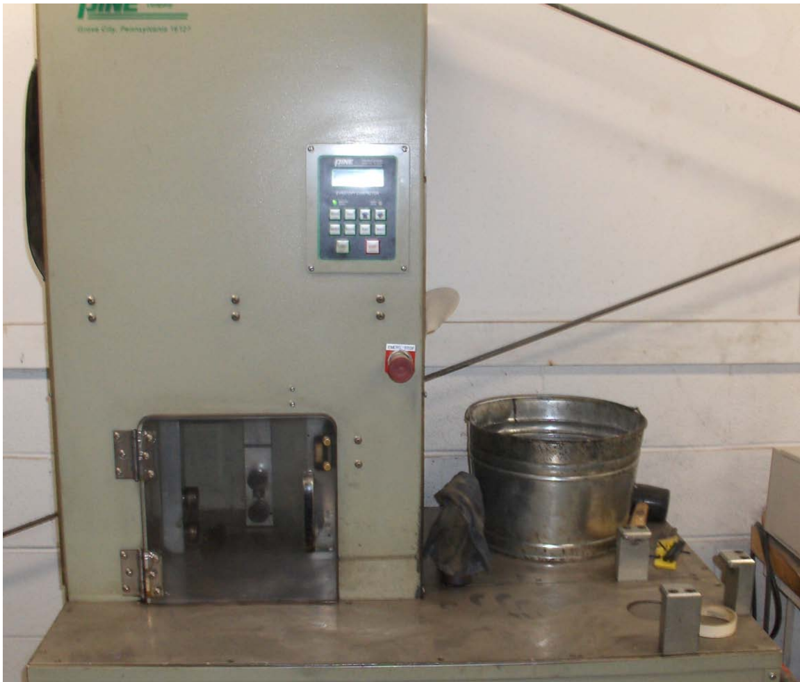
Figure 4-7. SUPERPAVE Gyratory Compactor Used in Laboratory Study.
