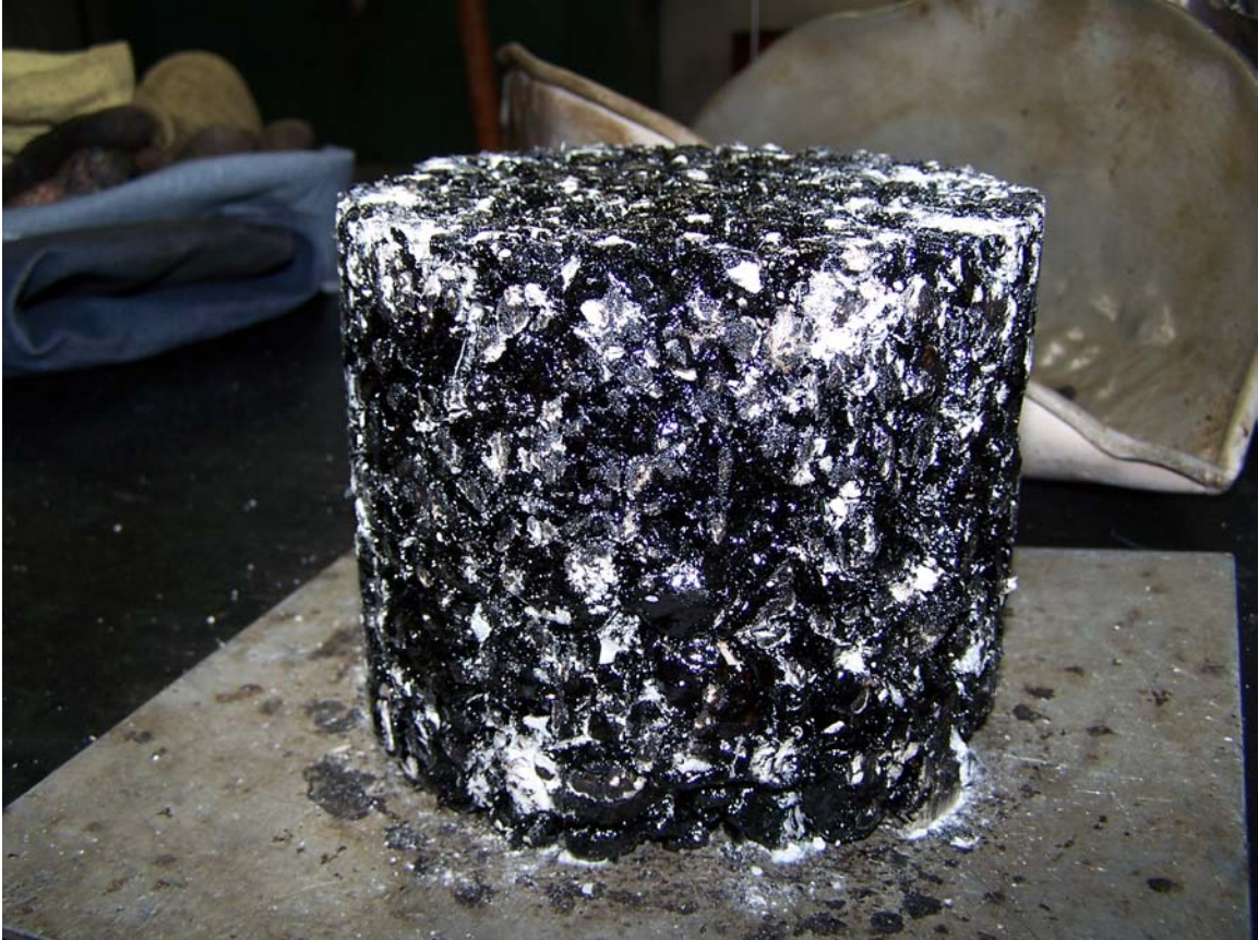
Figure 4-8. Aggregate Crushing in PATB Pill after 40 Revolutions.
