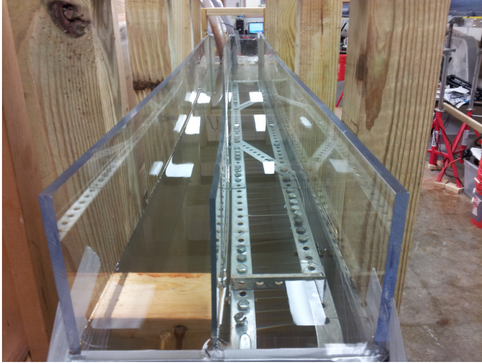
Figure 4.4: Longitudinal view from the downstream end of the acrylic tank with two settlers (lamella settler is in the right). Forebay is located in the opposite end
