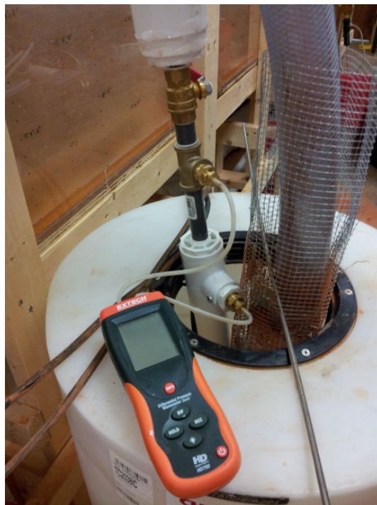
Figure 4.2 : Pressure-differential flow meter used to measure sediment-laden flows into the acrylic tank
