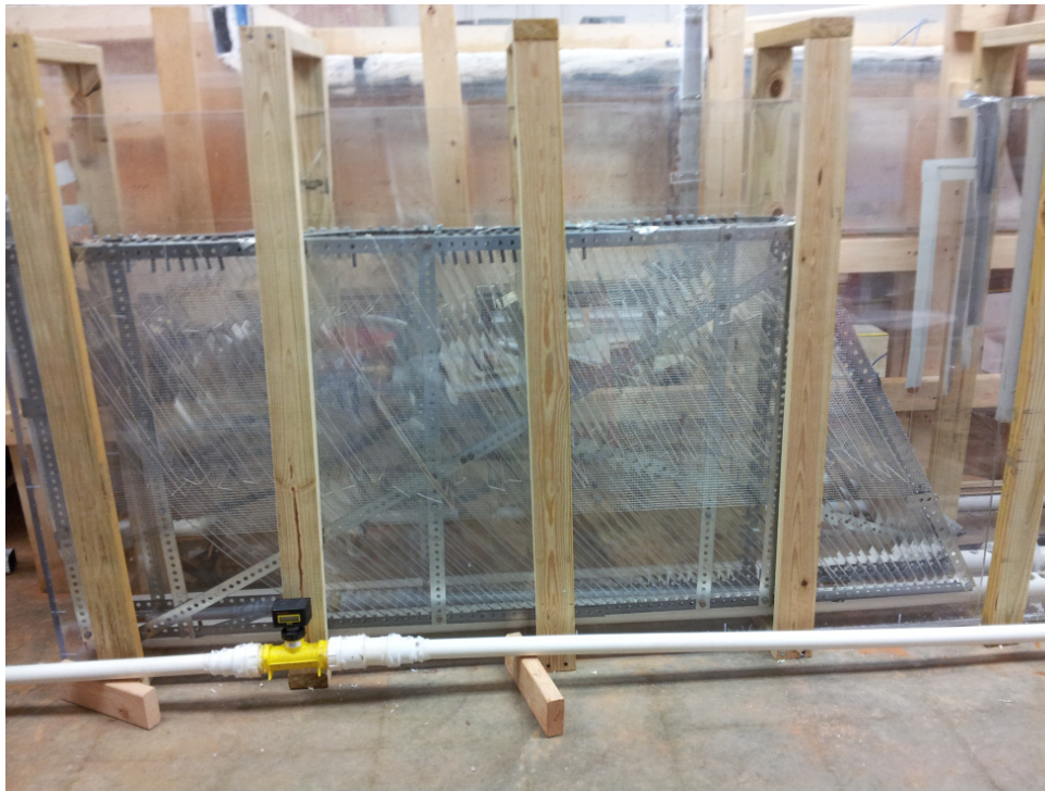
Figure 4.3: Lateral view of the acrylic tank (lamella settler in front). Forebay is located at the right end of the figure, and settled flow discharged at the left end of the system
