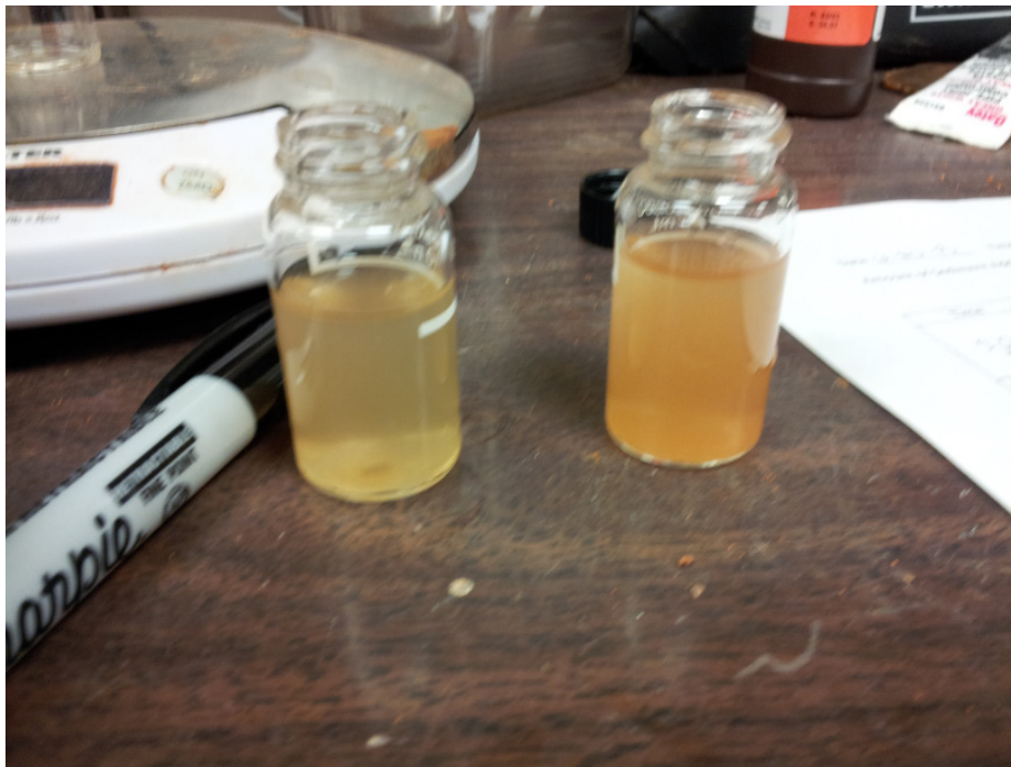
Figure 5.8: Samples collected at the outflow points of the lamella settling unit (left) and the traditional (control) settling unit.
