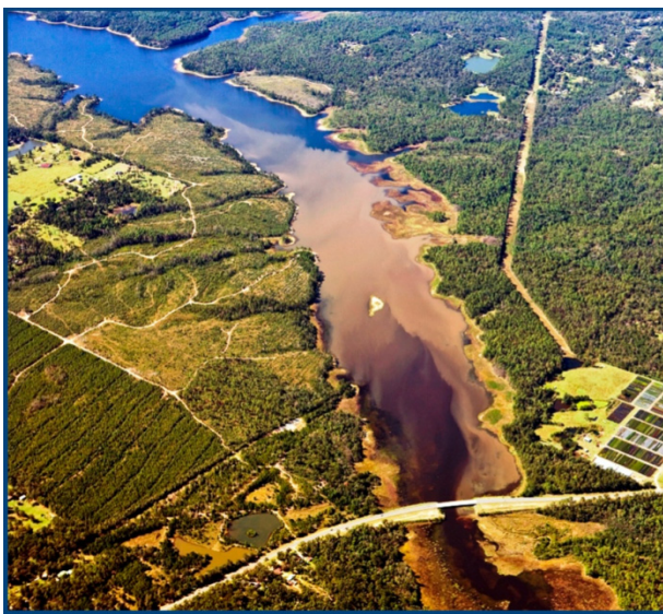
Figure 1.1 : Sediment plume resulting from road construction runoff (Clark et al. 2012)
