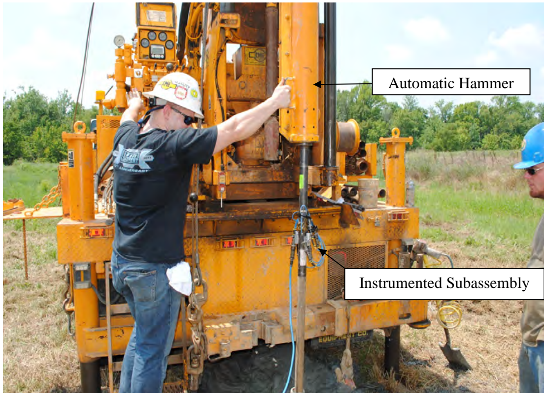
Figure 4.7 Final instrumentation setup prior to testing
