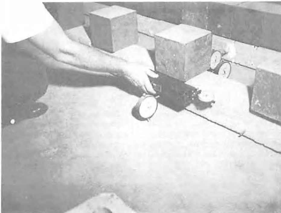
Fig. 5--View showing close-up of Whittemore gage and dial gage
