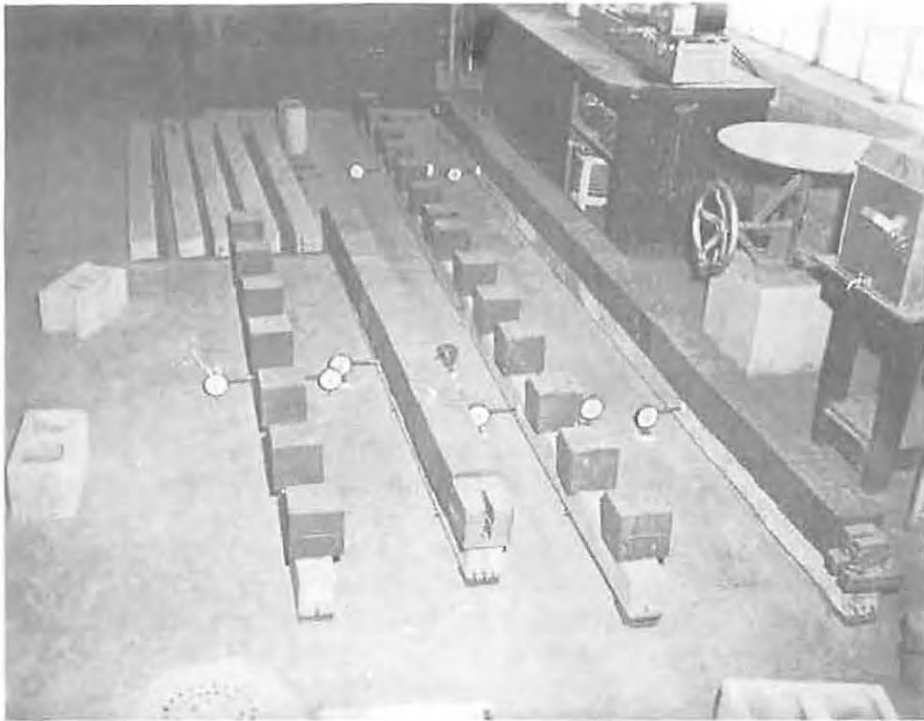
Fig. 4--View of test beams, shrinkage specimens and instrumentation
