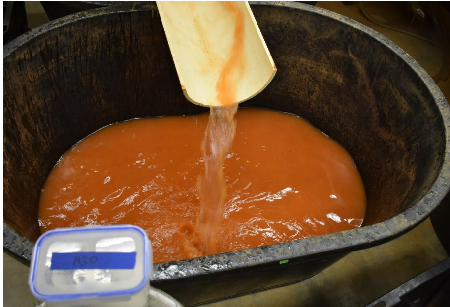
Figure 3.36: Flocculating Runoff Storage Tanks.
