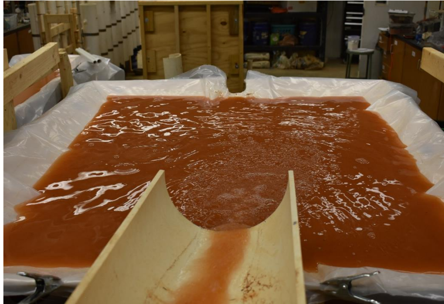
Figure 3.30 Undersized Basin: No Energy Dissipation or Skimmer.
