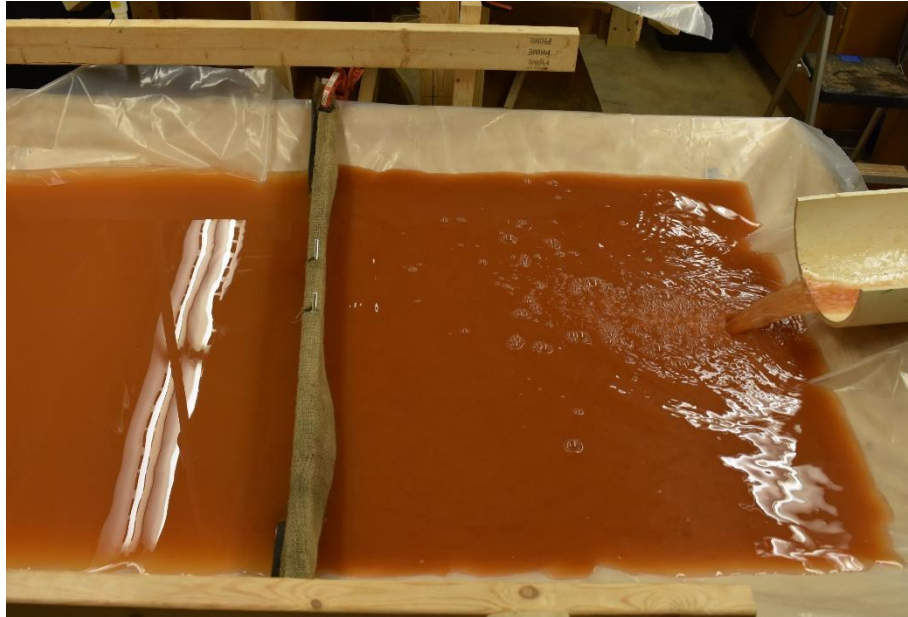
Figure 3.26: In-Channel Basin: Single Coir Baffle.
