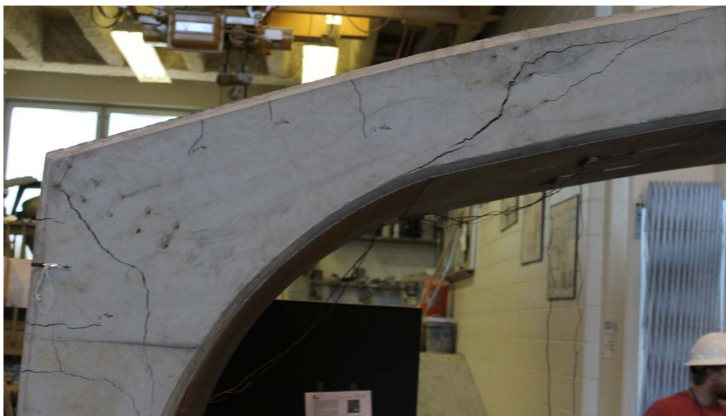
Figure 3-12 Corner Crack Immediately Prior to Failure
