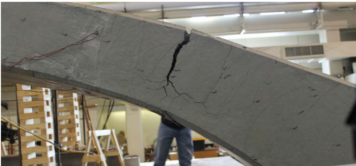
Figure 4-12 Bridge Section Immediately After Failure
