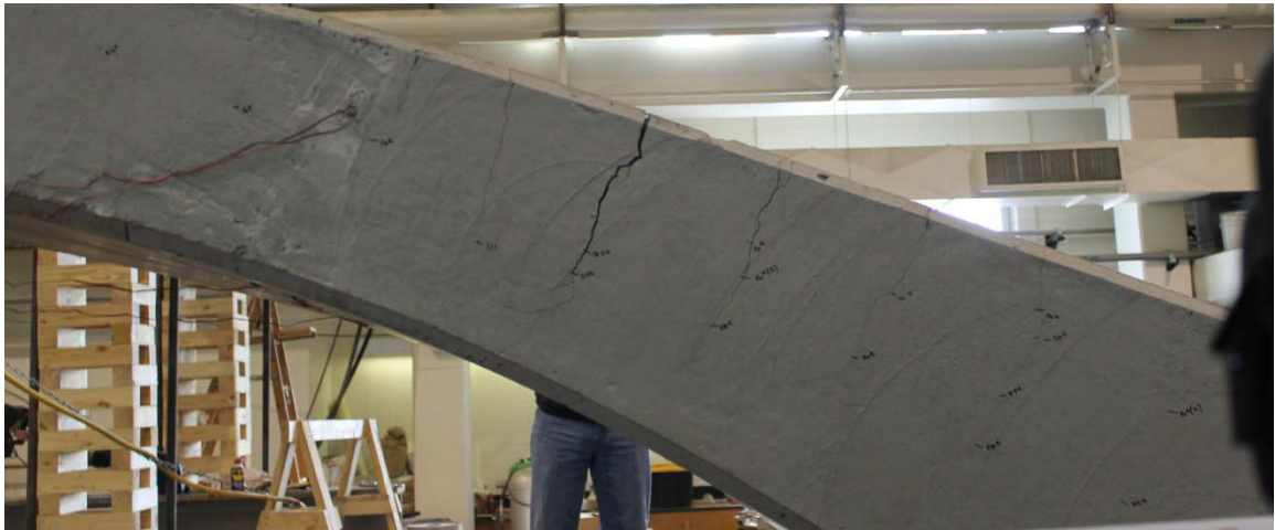
Figure 4-11 Bridge Cracking Immediately Prior to Failure
