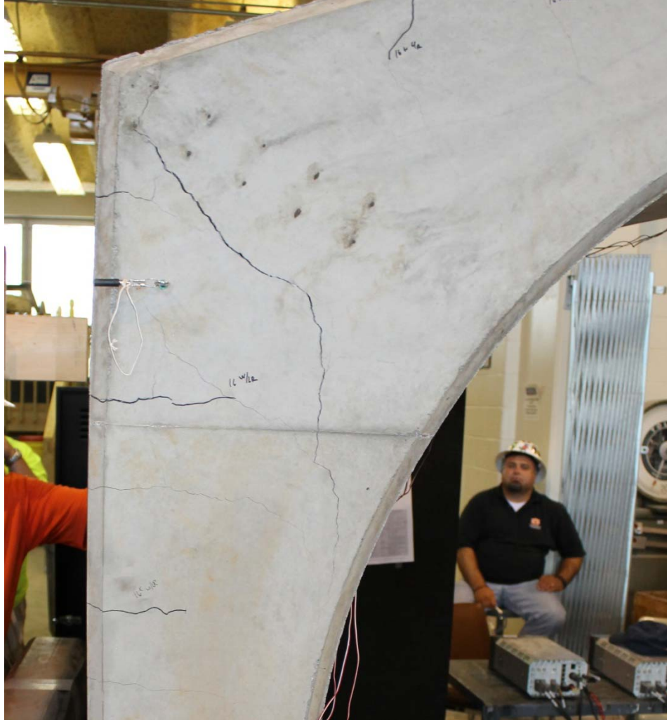
Figure 3-10 Corner Crack at 156 kips Total Load
