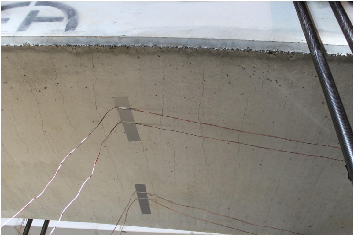
Figure 4-10 Midspan Cracking – 120 kips Total Load
