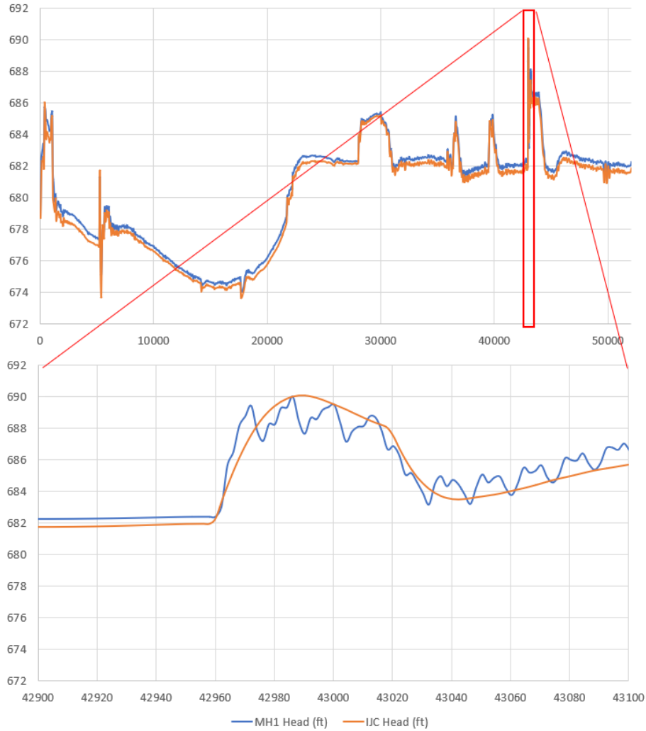
FIG. 27. Comparison of head elevation between IJC and MH1 for a scenario where there is a 12-in ventilation tower at MH1.
